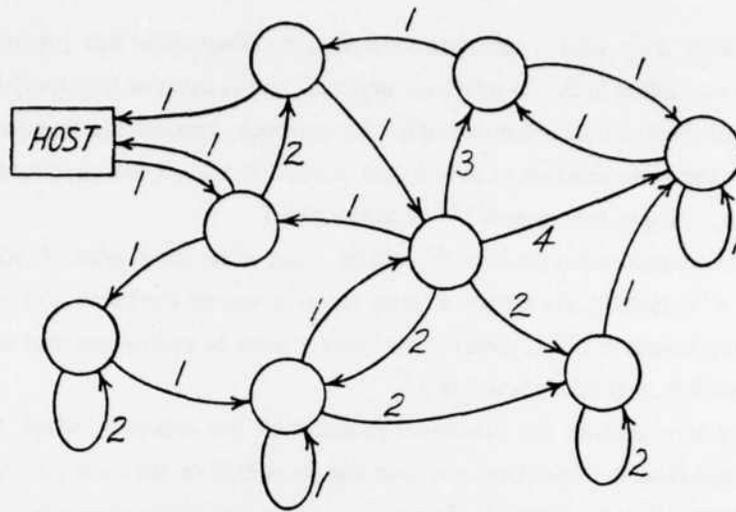
Figure 4: The systolic system  $S_3$  produced by applying the Systolic Conversion Theorem to the system  $S_1$  from Figure 1. Each edge  $(u, v, w)$  from  $G_1$  has been replaced by the edge  $(u, v, w + lag(v) - lag(u))$ , where the lag of a vertex is taken as the weight of the shortest path from that vertex to the host in  $G_1 - 1$  as indicated in Figure 3.
