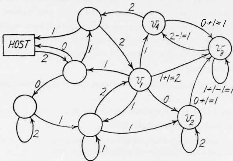
Figure 2: The communication graph of a system  $S_2$  which is equivalent to the system  $S_1$  from Figure 1 as viewed from the host. Internally, the two systems differ in that vertex  $v_3$  lags by one clock tick in  $S_2$  with respect to  $S_1$ .
