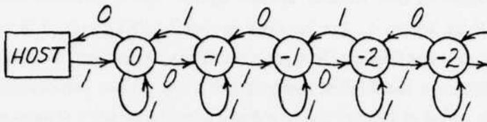
Figure 15: Communication graph of an optimized simulator for the real-time palindrome recognizer  $P$  of Figure 7. In the optimized simulator, no signal propagates through more than two functional elements in one clock period. Each vertex is labeled with its lag in this system with respect to  $P$ .
