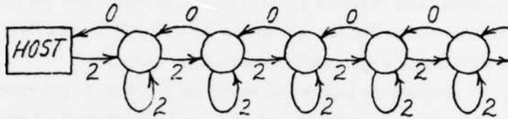
Figure 10: The communication graph  $2G$  for a 2-slow simulator  $2P$  of the system  $P$  from Figure 7. This graph is obtained by doubling the weight of every edge in the communication graph  $G$  of  $P$ .
