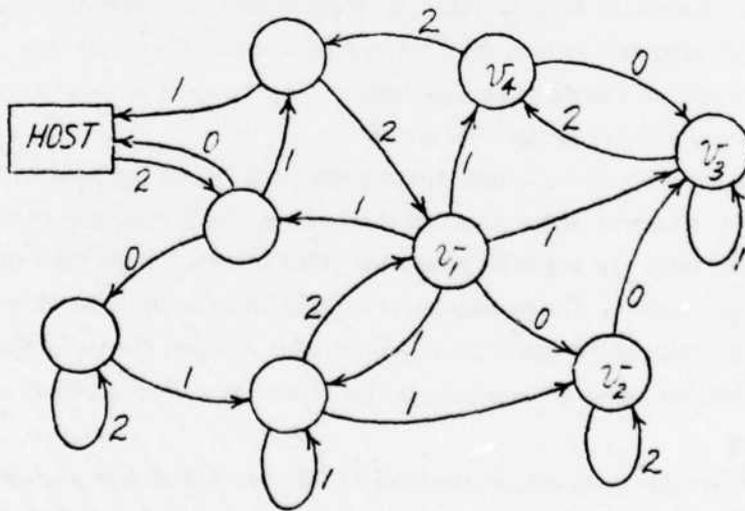
Figure 1: The communication graph  $G_1$  of a synchronous system  $S_1$ . One vertex of the graph is distinguished as representing not an ordinary functional element but a *host processor*, which is the system's only interface to the external world.
