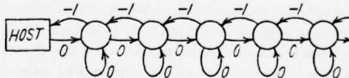
Figure 9: The constraint graph  $G-1$  for the real-time palindrome recognizer P from Figure 7. Since this graph contains cycles of negative weight, the Systolic Conversion theorem is not applicable to P.
