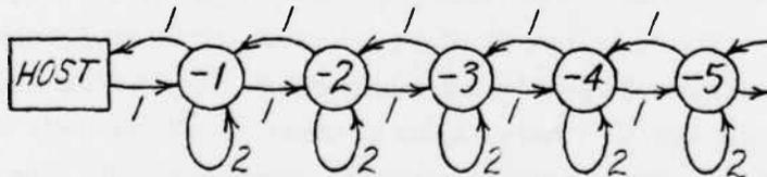
Figure 12: The communication graph of a systolic 2-slow simulator  $SP$  of the real-time palindrome recognizer  $P$  of Figure 7. Each vertex is labeled with its lag in  $SP$  with respect to the system  $2P$  shown in Figure 10.
