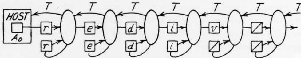
Figure 8: The configuration of the system P from Figure 7 as it recognizes the palindrome "redivider".
