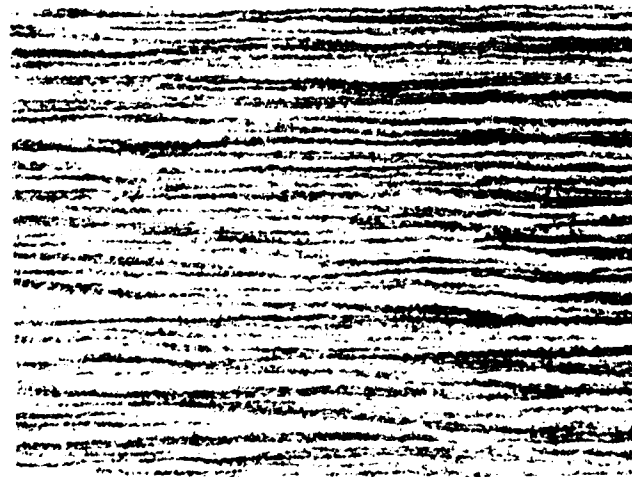
Figure 5. Banded structure of A1 material revealed by macro-etching with Oberhoffer's reagent.
