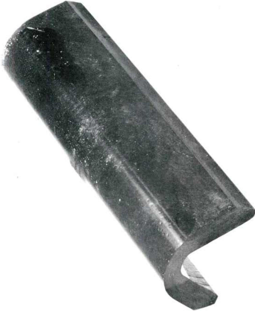
Figure 15 Creep Formed COMPGLAS™ Cylindrical Segment
