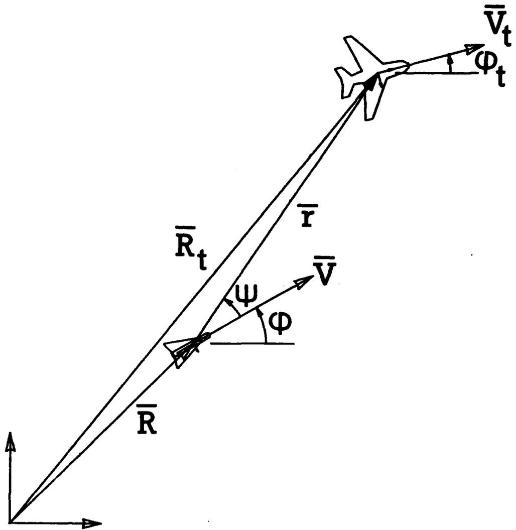
Figure 1. Geometry of interceptor and target.
