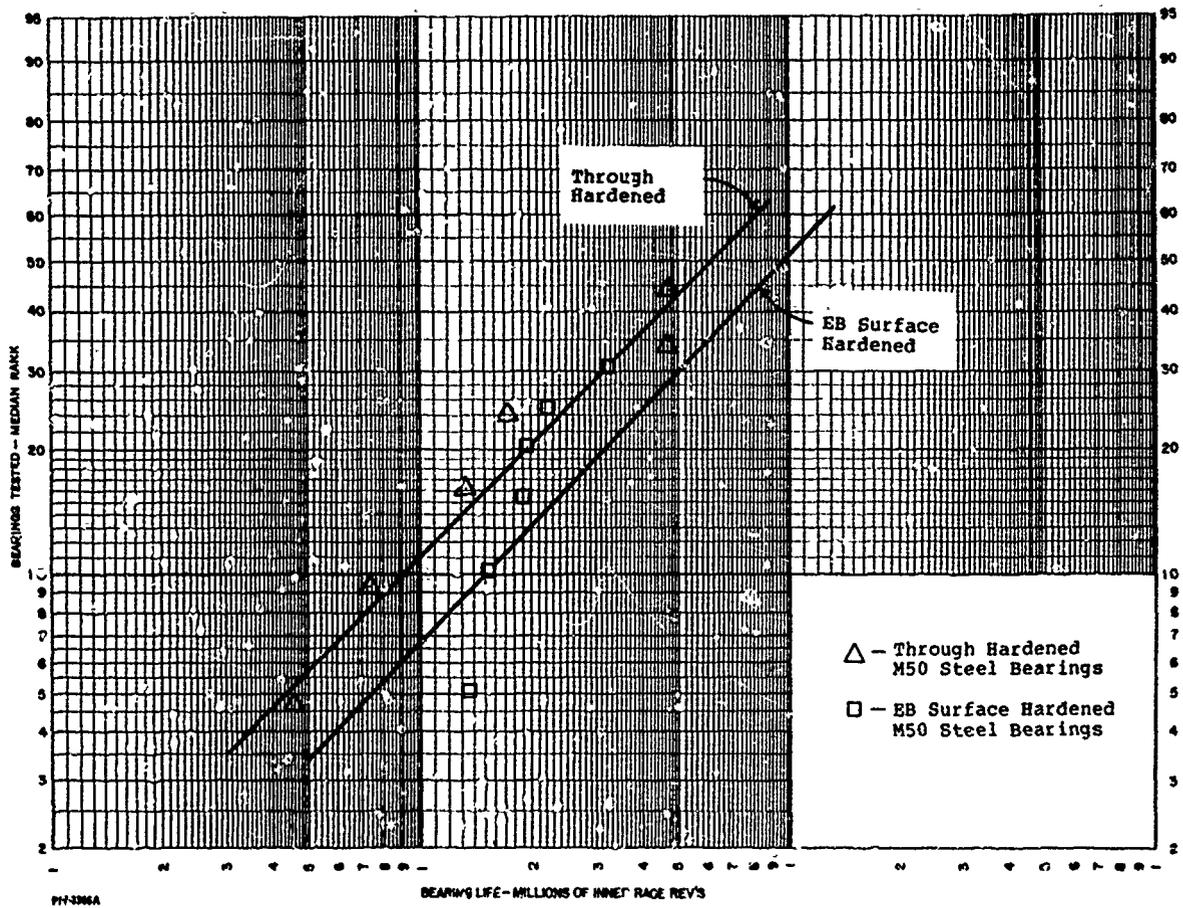
Figure 5. Weibull Plots of Through Hardened and EB Surface Hardened M50 Steel Bearing Life Data
