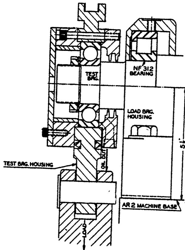
Figure 3. R2 Type Bearing Test Machine
