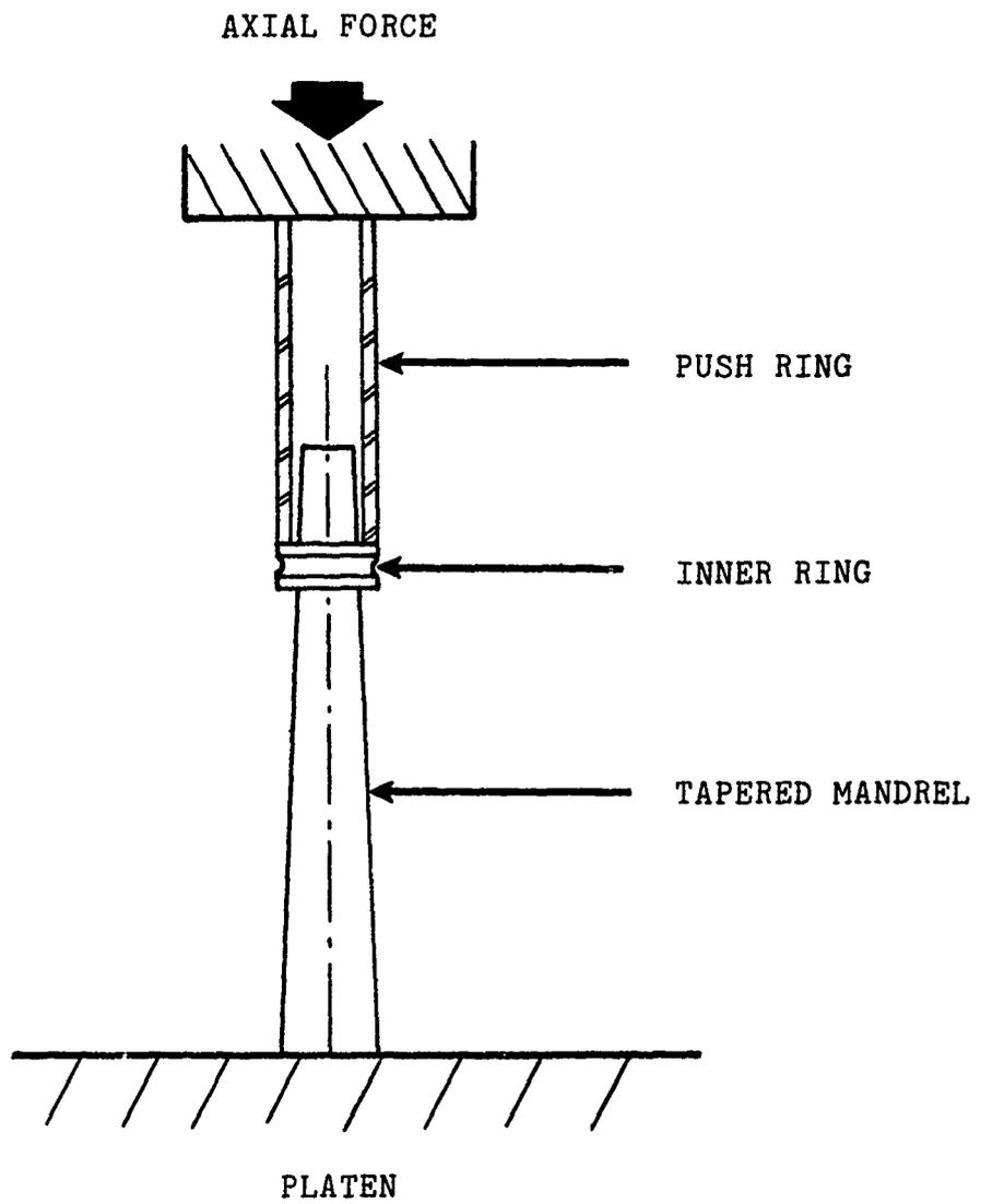
Figure 4. Apparatus for Radial Expansion of Bearing Inner Rings
