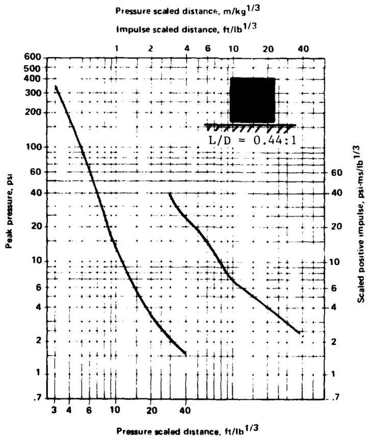
Figure 4. Pressure and impulse versus scaled distance for Cyclotol 70/30, 13.61 kg (30 lb) charge in fiberboard shipping container
