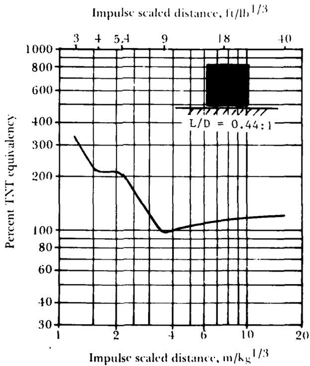
Figure 5. Pressure and impulse TNT equivalency for 13.61 kg (30 lb) fiberboard shipping container
