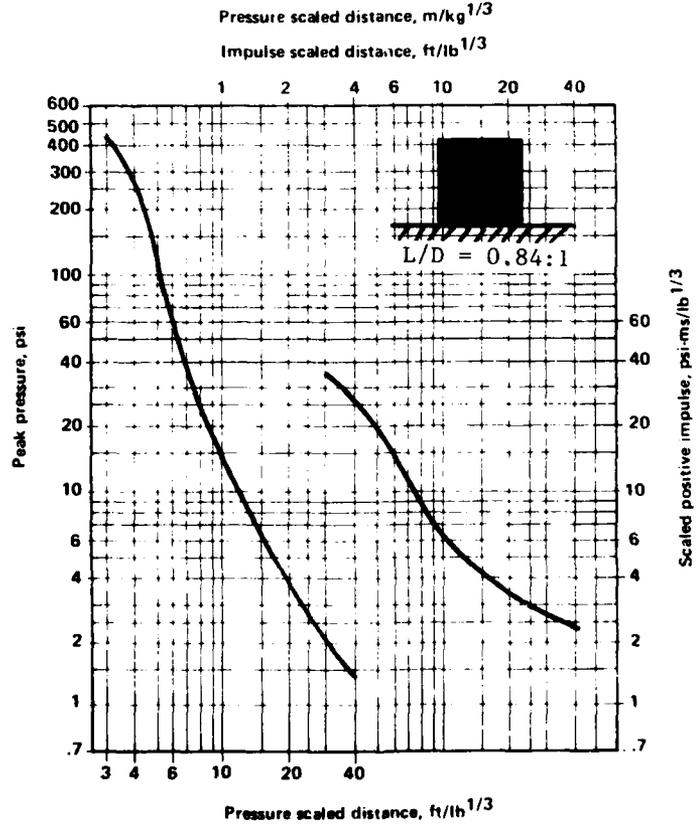
Figure 10. Pressure and impulse versus scaled distance for Cyclotol 70/30, 68.04 kg (150 lb) charge in fiberboard transfer box
