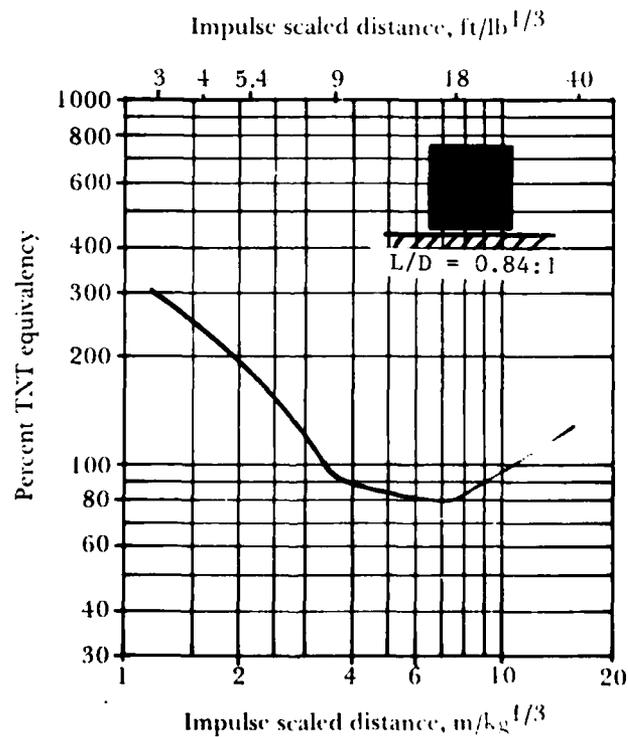
Figure 11. Pressure and impulse TNT equivalency for 68.04 kg (150 lb) fiberboard transfer box
