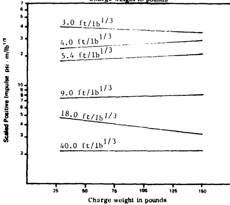
Figure 16. Deviation from cube root scaling
