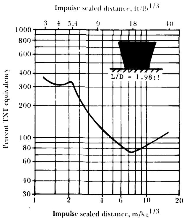
Figure 15. Pressure and impulse TNT equivalency for 68.04 kg (150 lb) simulated wood hopper
