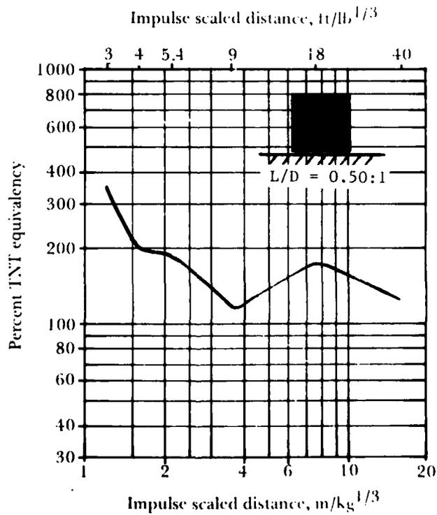
Figure 7. Pressure and impulse TNT equivalency for 27.22 kg (60 lb) fiberboard shipping container
