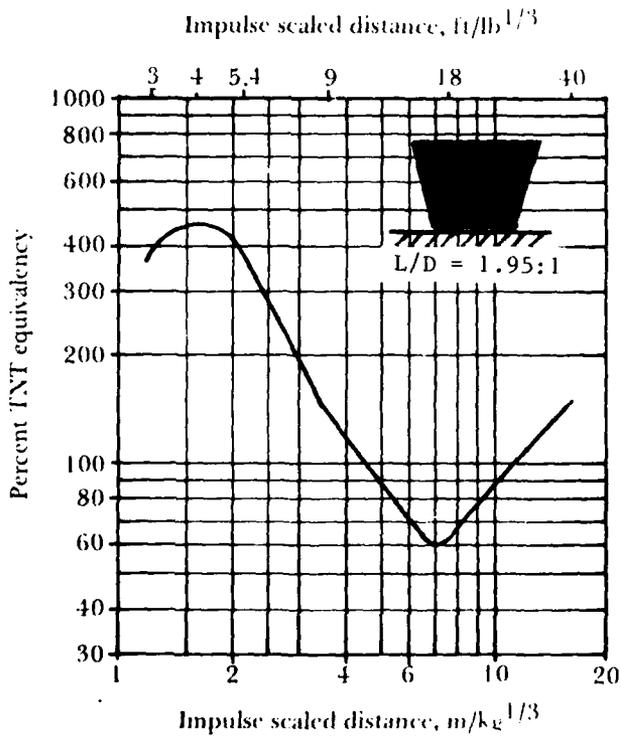
Figure 13. Pressure and impulse TNT equivalency for 45.36 kg (100 lb) simulated wood hopper
