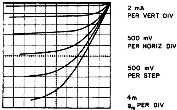
FIGURE 16. P-CHANNEL DRAIN CHARACTERISTIC OF DEVICE FABRICATED AT SANDIA LABORATORIES
