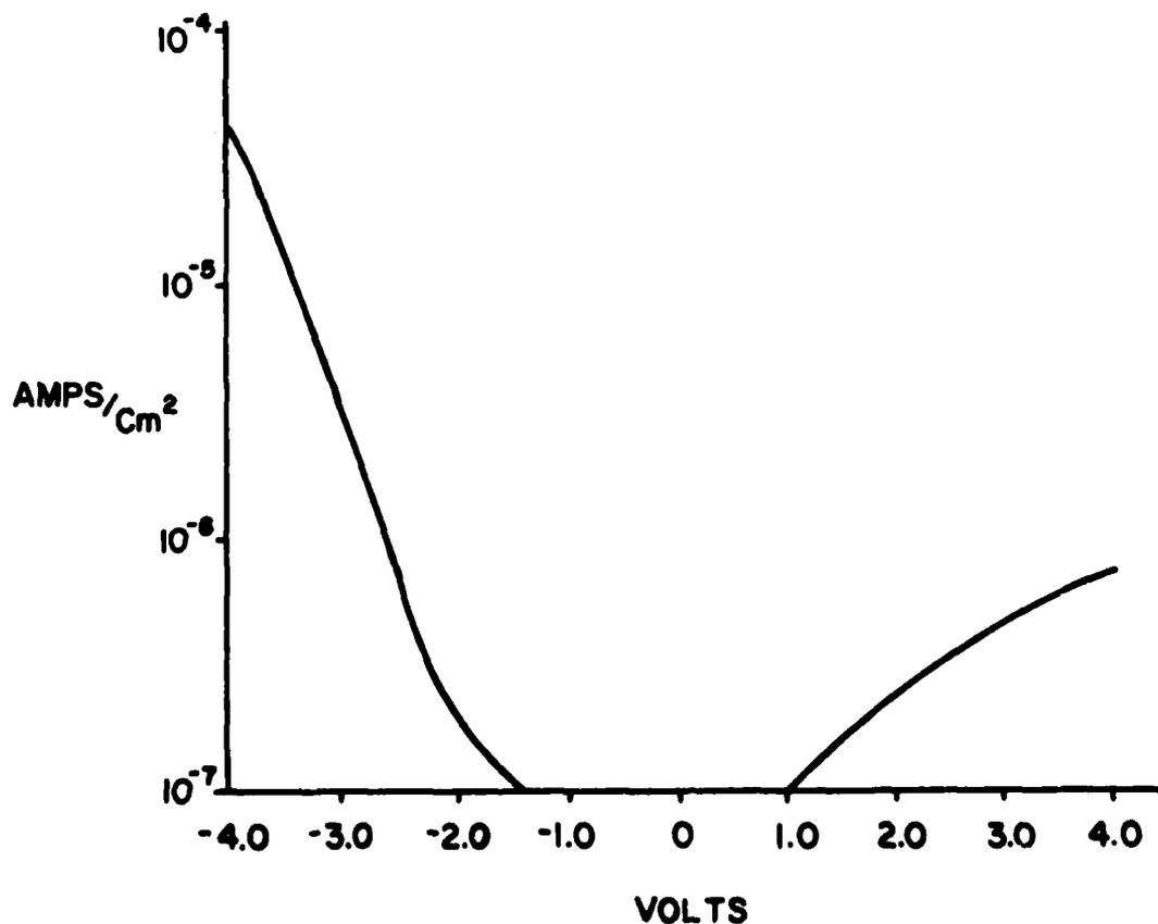
FIGURE 13. I-V CHARACTERISTIC OF FILM ON P-TYPE SILICON
