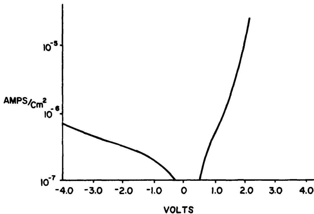
FIGURE 12. I-V CHARACTERISTIC OF FILM ON N-TYPE SILICON
