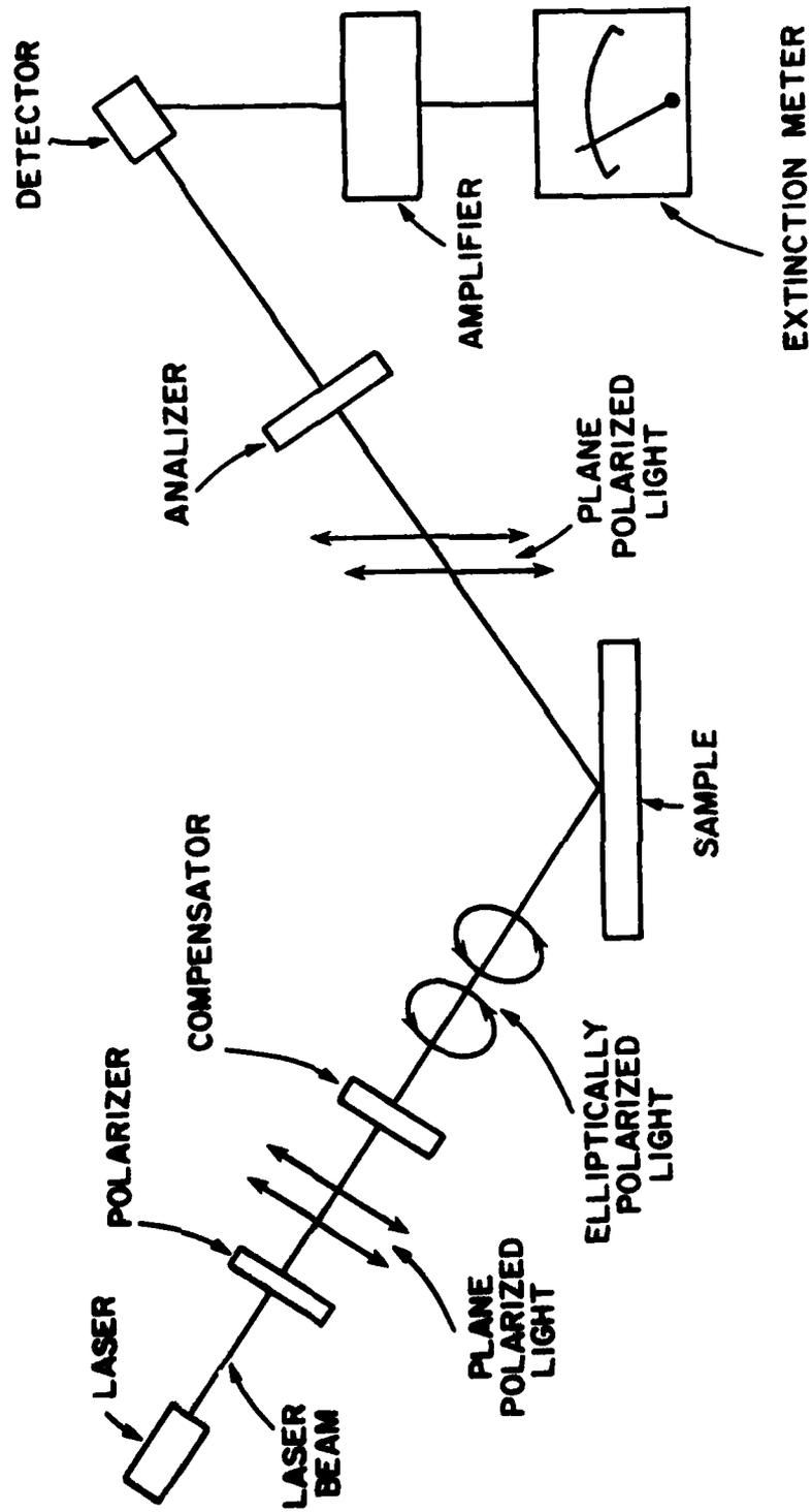
FIGURE 3. SCHEMATIC DIAGRAM OF ELLIPSOMETER
