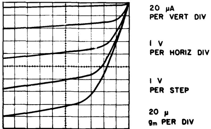
FIGURE 18. DRAIN CHARACTERISTIC OF A 2  $\mu$ m LONG RI TRANSISTOR
