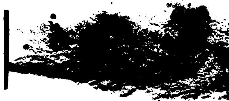
Fig. 5.28. Schlieren photograph taken at the onset of the almost "continuous popping sound" state of cavity development in the 6.35mm jet at  $Re_D = 1.29 \times 10^5$  and  $\sigma = 0.19$ .
