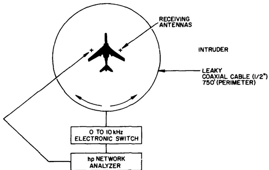
Figure 12. Single Wire Individual Resource Protection Sensor (Switching)
