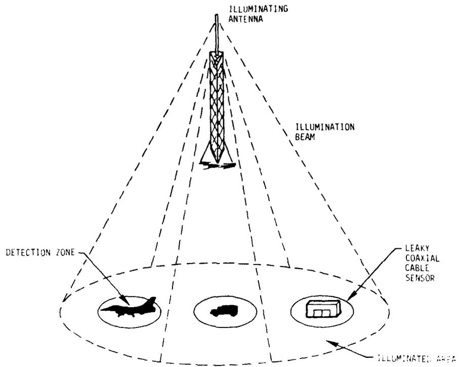
Figure 1a. Illumination Detection System for Small Areas
