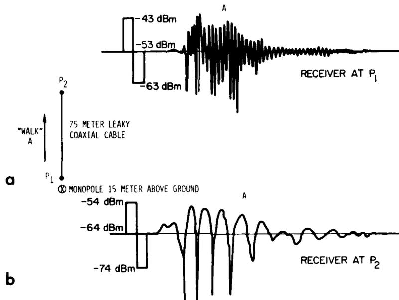
Figure 10. Power Received from One End of Leaky Coax Cable (Monopole Height = 15 m)
