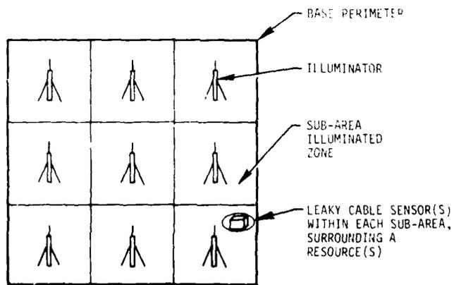
Figure 1b. Illumination Detection System for Large Areas
