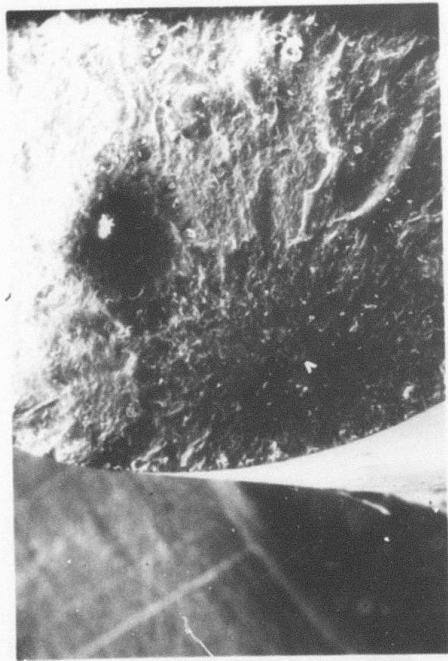
a) General area showing fracture mirror v, indicates origin 35x
