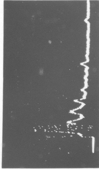
b) Fracture mirror & origin origin indicated by, v, 45x
