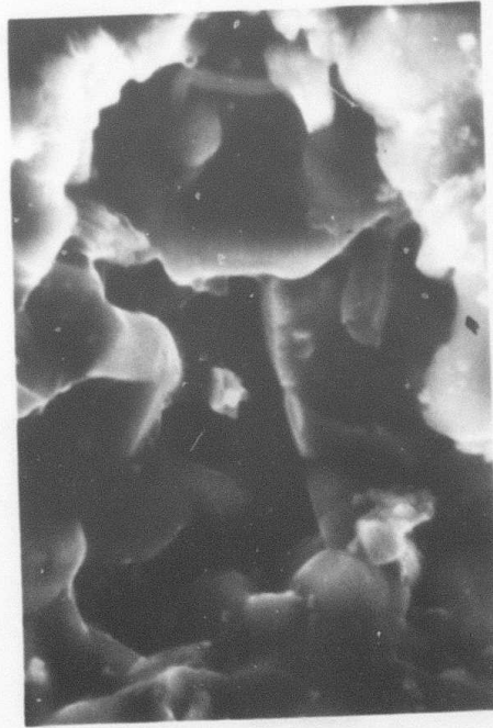
a) General area showing fracture mirror v, indicates origin 35x
