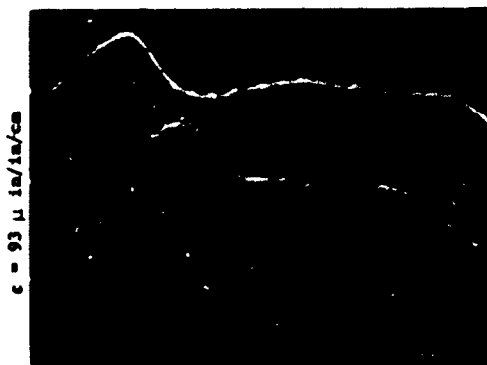
Figure 13. Strain Pulse Propagating in an 0.75 inch Diameter Concrete Bar (Ball, 204 in/sec, u, A-3, 28, 20 μ sec/cm, 0.2 m volt/cm.)
