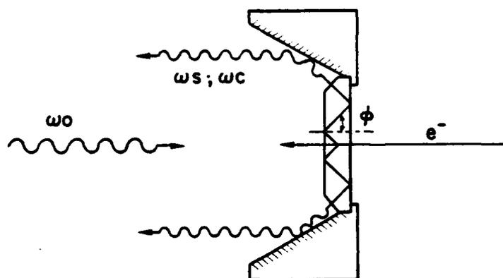
Fig. 2 - The target/mirror combination. The mirror diameter is of the order of 1 inch.
