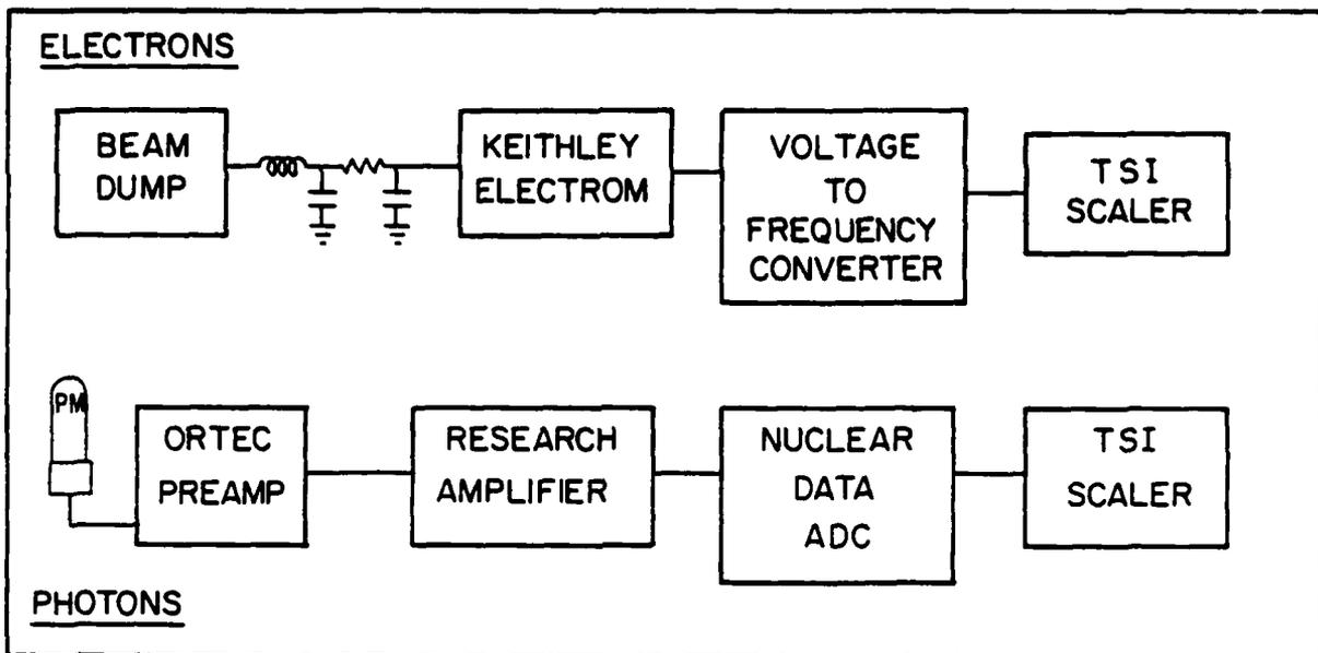
Fig. 6 - Block diagram of data collection system
