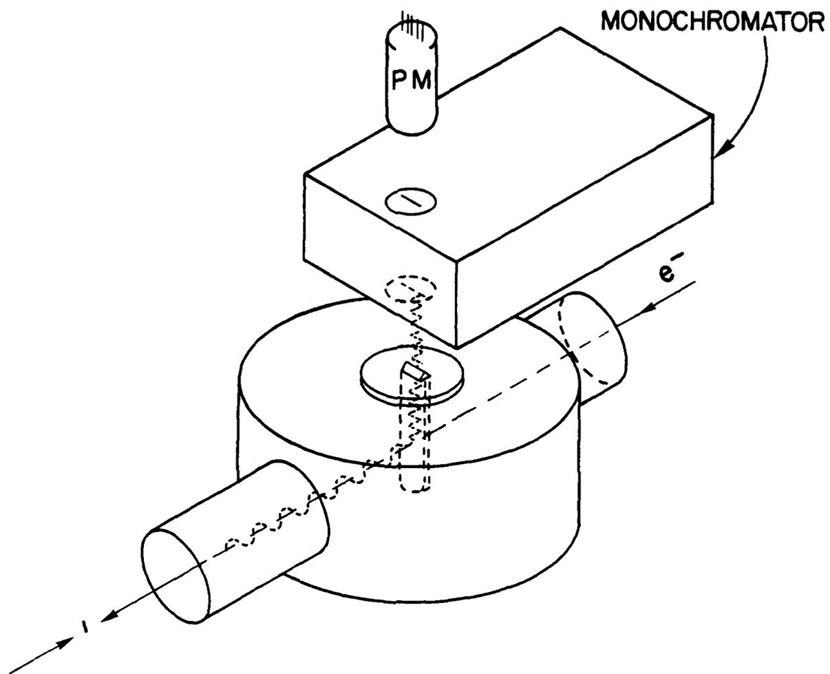
Fig. 5 - Layout of target chamber and monochromator
