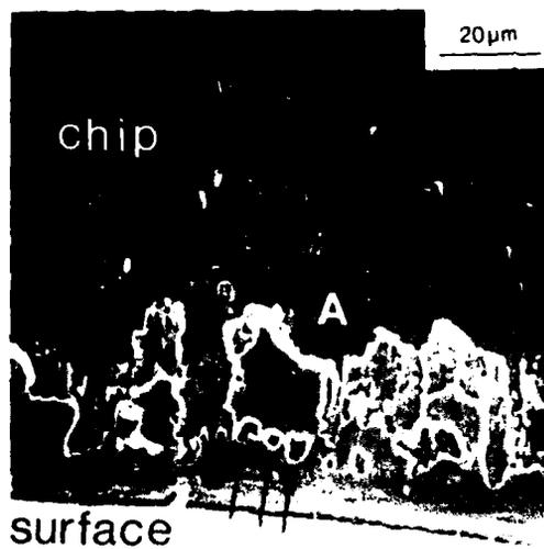
FIG. 7 Scanning electron micrograph at the chip root of the rake face side of a chip. There is a "smooth region" at the chip root in which there are some holes (arrowed) where metal has been removed. Further away from the chip root (region A) metal has been completely removed.
