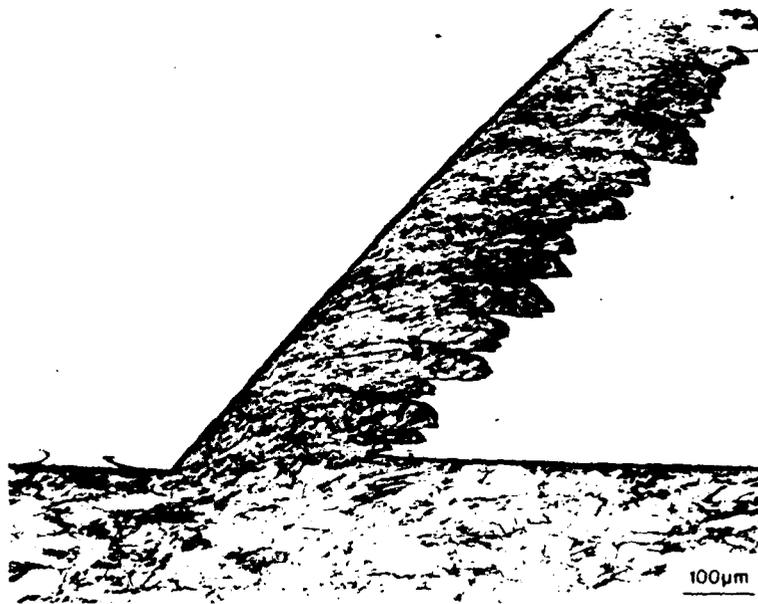
FIG. 4 Optical micrograph of a mid-section of an interrupted cut made with a cutting tool of  $-40^\circ$  rake angle. Note that the deformation within the chip is relatively uniform (cf. Fig. 2). Cutting speed  $2.5 \times 10^{-2}$  m/s.
