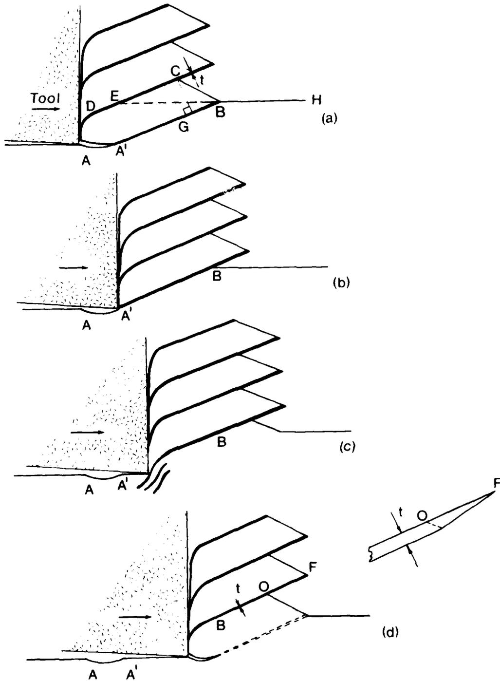
FIG. 3 Diagrammatic illustration of the steps involved in the formation of a segment.
