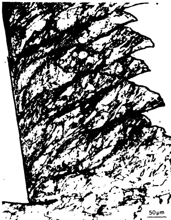
FIG. 2 Optical micrograph of a mid-section of an interrupted cut showing that the deformation is concentrated between the segments in very narrow shear bands. Depth of cut  $150\ \mu\text{m}$ ,  $+10^\circ$  rake angle, cutting speed  $2.5 \times 10^{-2}$  m/s.
