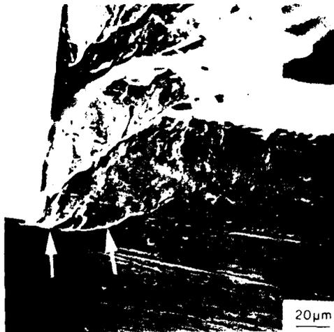
FIG. 1 Scanning electron micrograph of an interrupted cut (in air). Distinct segments are present and a crack (arrowed) can be seen running into the chip adjacent to the cutting edge.
