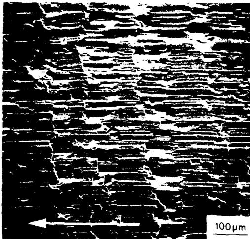
FIG. 12 Scanning electron micrograph of a machined surface showing rows of fracture separated by relatively smooth regions. Depth of cut  $125 \mu\text{m}$ ,  $+10^\circ$  rake angle. The arrow indicates the direction of cutting.
