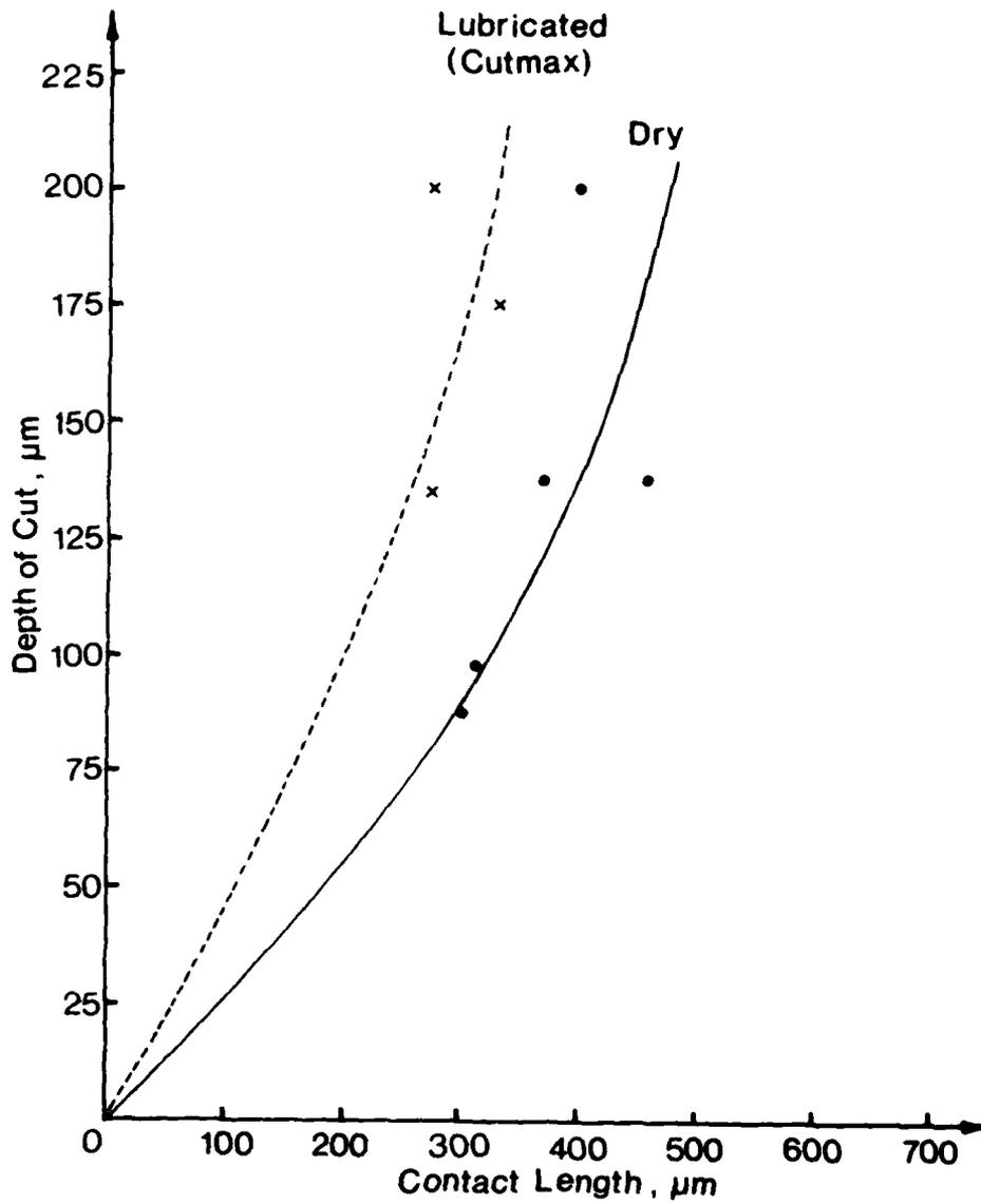
FIG. 11 Effect of machining with a neat cutting oil on the relation between depth of cut and contact length. Rake angle + 10°, cutting speed  $2.5 \times 10^{-2}$  m/s.
