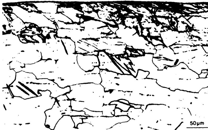
FIG. 16 Optical micrograph of a normal section through a machined surface showing that a deformed layer containing many deformation twins is present. Note the fragmented layer which occurs right at the surface is too shallow in this case to be observed.
