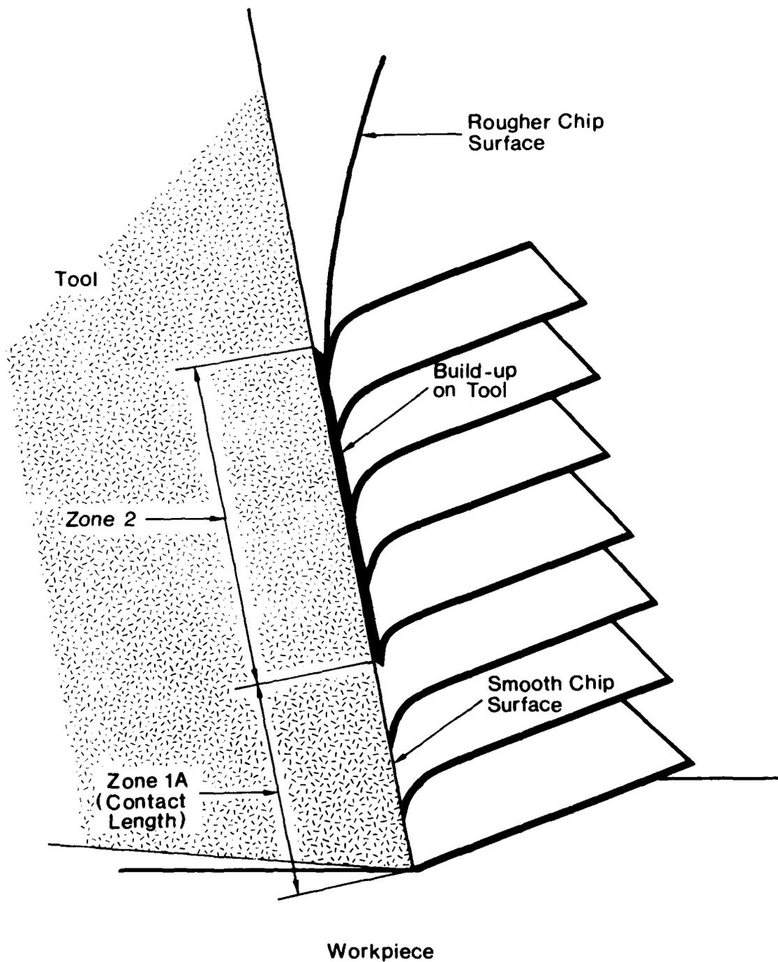
FIG. 9 Schematic sketch of the tool/chip interactions.
