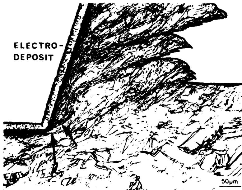
FIG. 15 Optical micrograph of a mid-section of an interrupted cut. Shear bands in the chip (arrowed) can be seen bending around the cutting edge into the machined surface. Depth of cut  $125\ \mu\text{m}$ ,  $-20^\circ$  rake angle, cutting speed  $2.5 \times 10^{-2}$  m/s.
