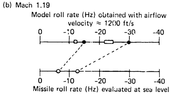
Fig. 2 Model roll rates tested and equivalent missile roll rates.
