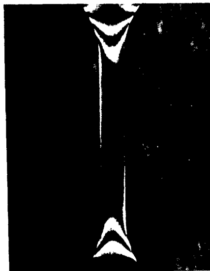
Fig. 4 Stress Field by Photoelastic Technique (Plane Polarized) of Routinely Mounted Specimen. Load Approximately 57 lbs. ( \sigma = 1824 psi)
