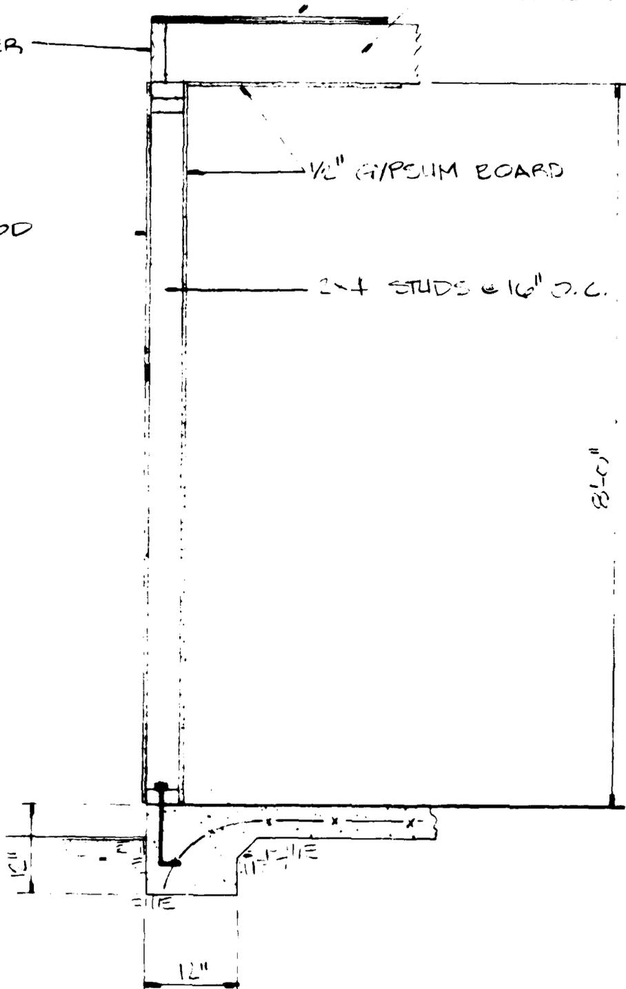
Fig. 2-4. Section Through Exterior Wall, DNA No. 5001.
