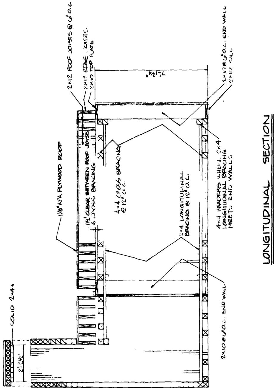
Fig. 8-4. Longitudinal Section Through Shelter.
