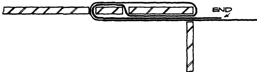
Fig. 7-12. Sketch of Soil Anchor/Webbing Arrangement.
