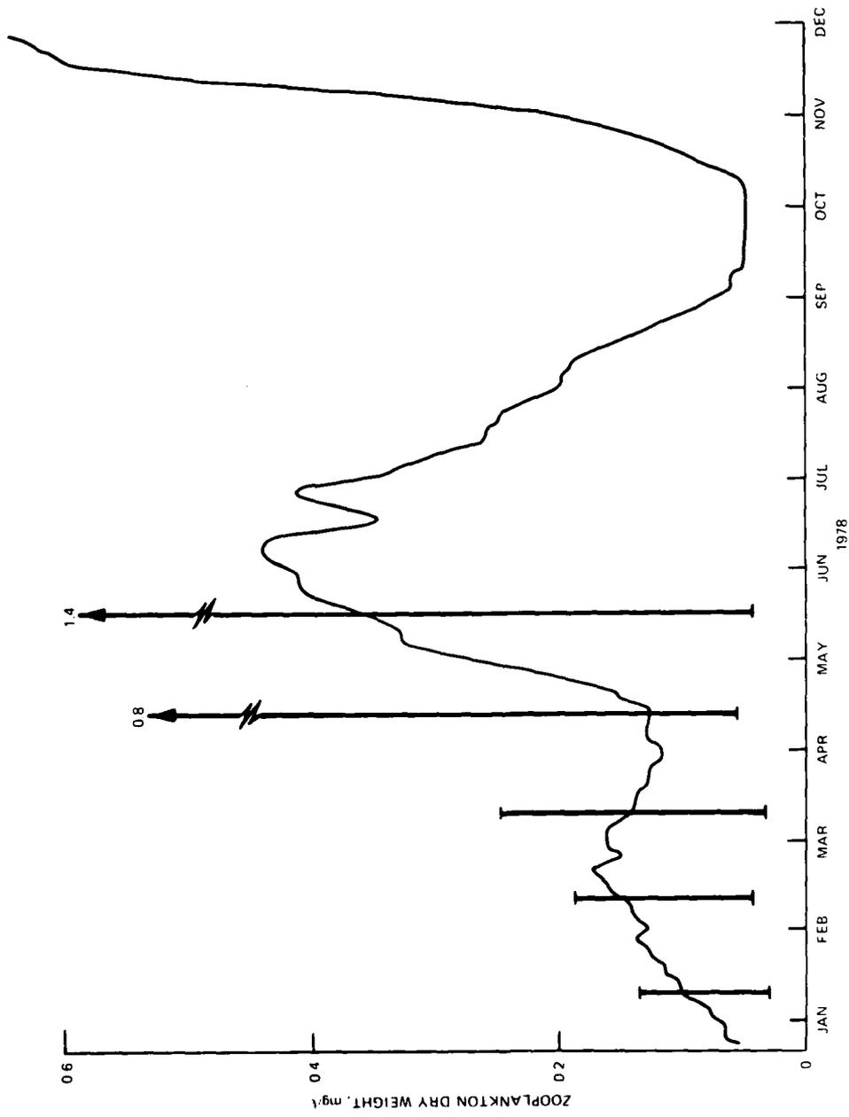
Figure 6. Simulation of zooplankton in the surface layer. Vertical bars represent minimum and maximum measured values
