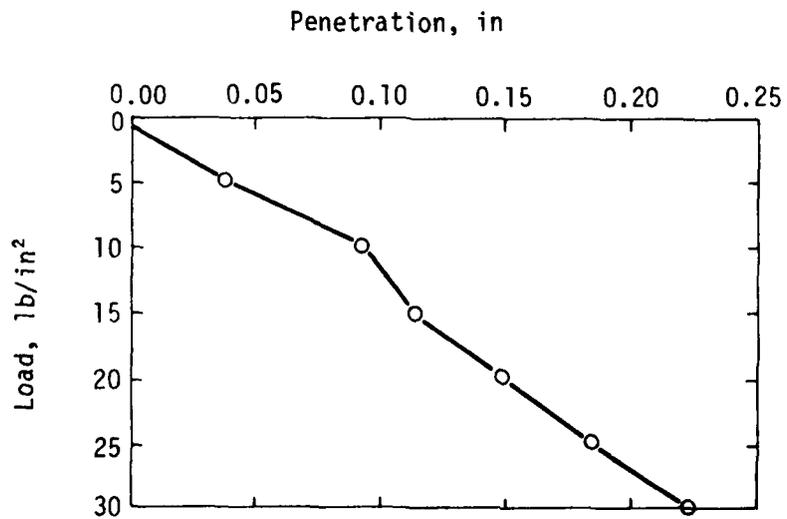
Figure 6. Plate bearing on crushed limestone material.
