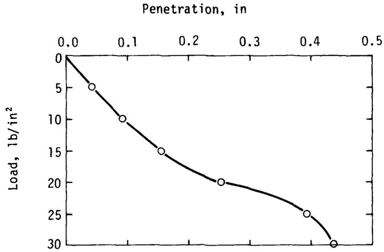
Figure 5. Plate bearing on compacted pushback material.
