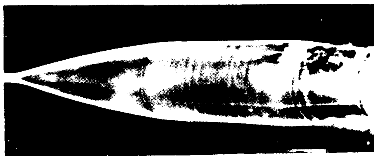
Figure 11b. Smoke Photograph for Re = 928,000 , 0 rpm, \alpha = 0^\circ .
