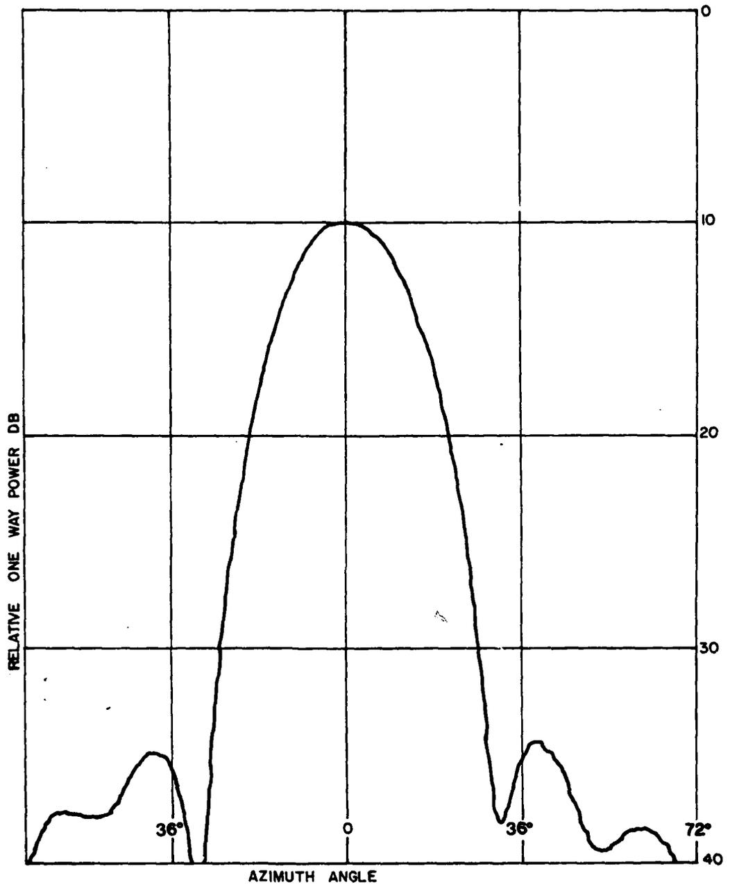
Figure 3.4 Azimuthal Antenna Pattern
