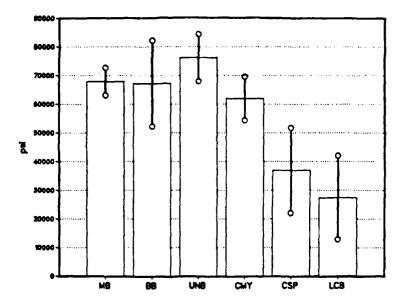
**TABLE 3.** MEANS AND STANDARD DEVIATIONS FOR ULTIMATE TENSILE STRENGTH VALUES.
