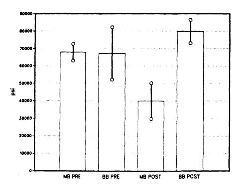
All of the solders tested yielded some solder joints with strengths exceeding those of conventional gold solder joints; however, some alloys had a large number of low strength joints. Difficulties were encountered soldering each of these non-precious alloys by the gas-oxygen torch method.
