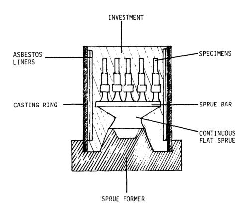
All casting was done on a centrifugal broken arm dental casting machine. The alloys were melted with a gas/oxygen flame using a multioriface tip as recommended by the manufacturer (KL-R Perplex, Perkeo Company, West Germany).
