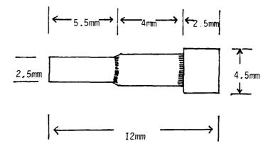
Figure 2. Cut Away Diagram of Casting Ring Showing the Position of the Specimen Patterns in the Ring Before Casting.
