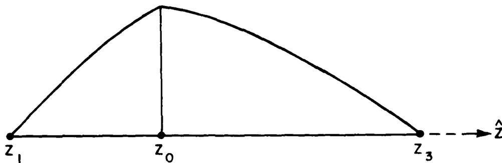
Figure 9. A linear test dipole and its sinusoidal current distribution. The endpoints are at z_1 and z_3 with terminals at z_0 .
