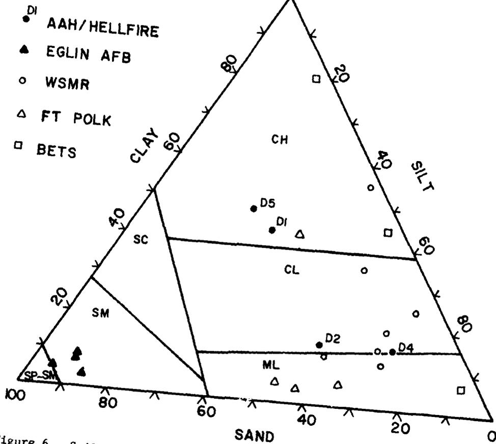
Figure 6. Soil classification chart showing locations of the Redstone samples together with data from other similar tests for comparison (Eglin AFB is the site of the Smoke Week II test (November 1978); WSMR is the site of the DIRT II test (July 1979); Ft. Polk is the site of the DIRT III test (April 1980). The BETS series consists of selected "tailored" soils and is being conducted at WES.)
