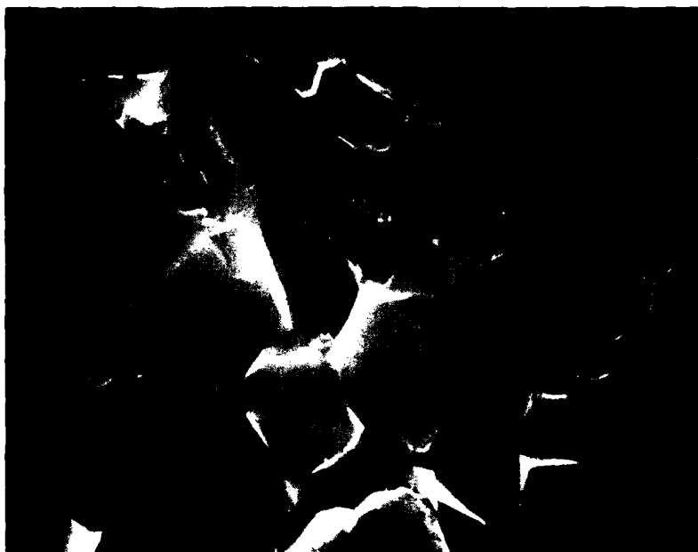
Figure 30. Area A fractured at K_I = 3-4 \text{ MPa m}^{1/2} showing mainly transgranular fracture (96% alumina Specimen #8, \sigma_F = 509 \text{ MPa} , 4000X).
