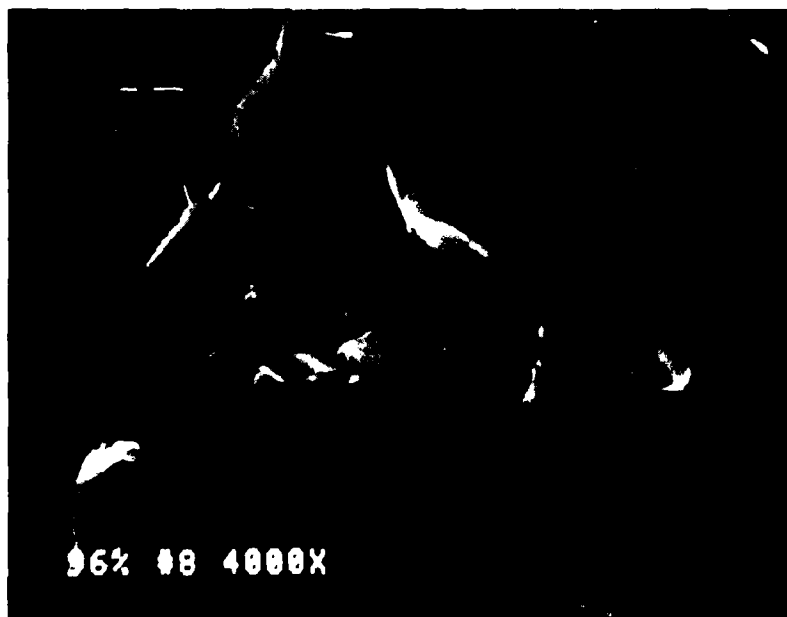
Figure 31. Area B fractured at K_I \approx 6.5 \text{ MPa} showing cleavage steps (96% alumina Specimen #8, \sigma_F = 509 \text{ MPa} , 4000X).
