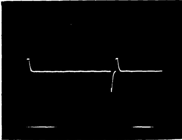
Figure 3.2.3.4-3. Helix Regulator Output (50V/cm, 20 ms/cm)
