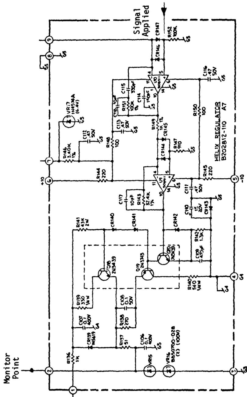
Figure 3.2.3.4-2. Helix Regulator Schematic
