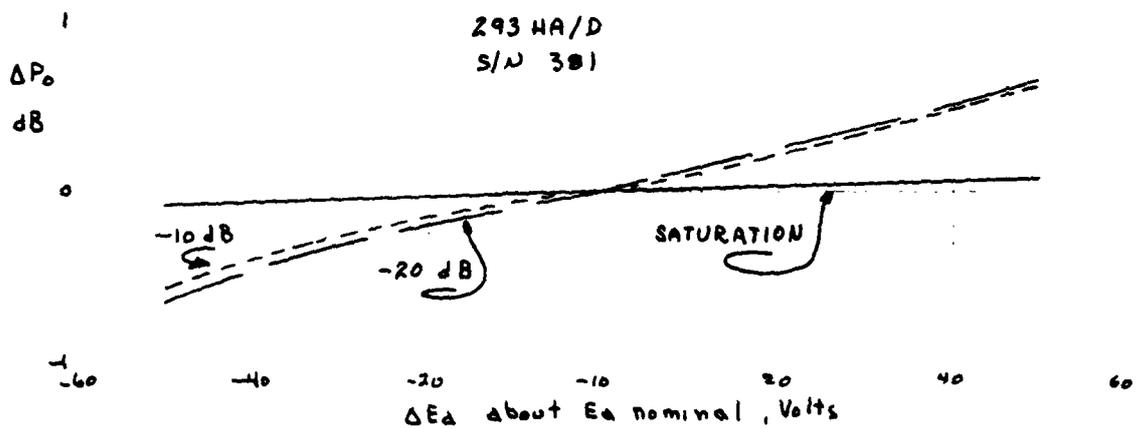
Figure 3.2.3.5-2. RF Power Output Variations About the Nominal Value For Three Levels of Power Output Vs Changes in  $E_a$
