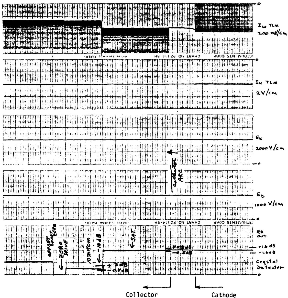
Figure 3.2.3.1-5. Collector Spark Strip Chart with Cathode Spark Data Comparison
