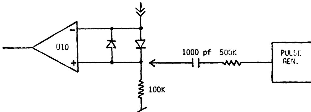
Figure 3.2.3.4-1. Helix Regulator Test Setup
