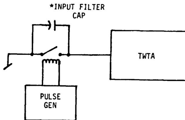
Figure 3.2.3.3-1. Shorted Filter Capacitor Test Configuration
