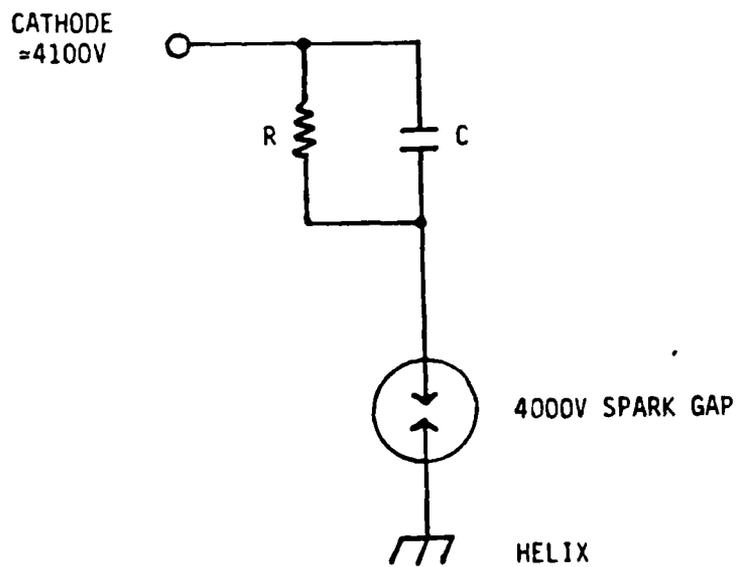
Figure 3.2.3.1-1 Spark Test Configuration
