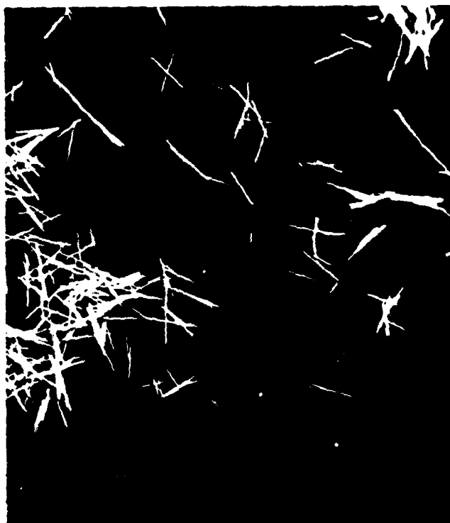
Figure 2. Transmission and scanning electron micrographs of cleaned \beta -FeOOH particles (K-115-1).
