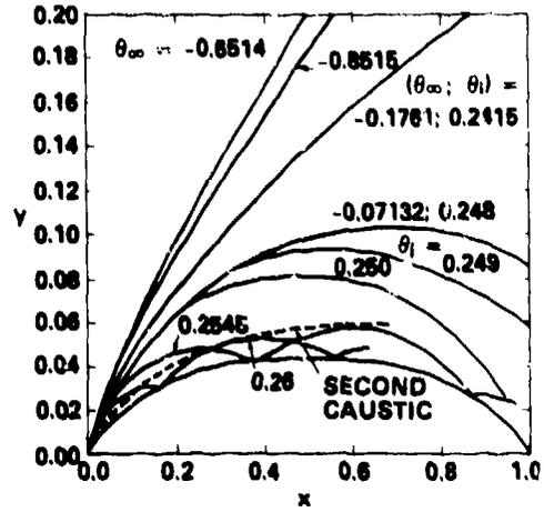
Figure 3 - Ray Paths for a Wigley Hull
