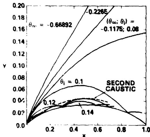
Figure 1 - Ray Paths for a Wigley Hull
