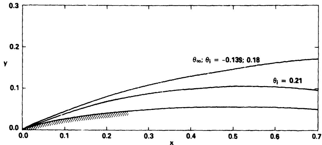
Figure 7 - Rays of the Wigley Ship ( $b = 0.2$ ,  $h = 0.0625$ ) with Bulb (radius,  $r_b = 0.0214h$ , depth,  $z_1 = 0.5h$ )
