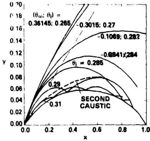
Figure 2 - Ray Paths for a Wigley Hull
