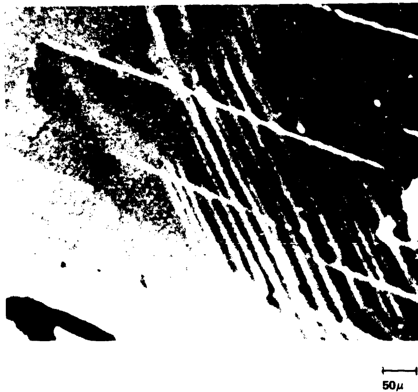
FIGURE 11 SCANNING ELECTRON MICROGRAPHS OF A Cu - 14.1 wt% Al - 3.0 wt% Ni ALLOY (B) AFTER STRESS-INDUCED MARTENSITIC TRANSFORMATION
