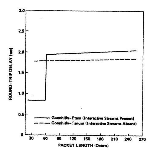
Round-Trip Delay as a Function of Packet Length Figure 2
