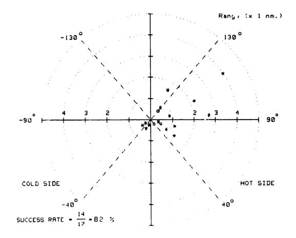
Figure 8. Sample display format for Envelope Recognition: Sidewinder AIM 9L -- shows fighter aircraft position at missile fire in terms of range (n.m.) and angle off tail (AOT in degrees) from target. Circles and stars indicate hits and misses, respectively, according to preselected rules for scoring.
