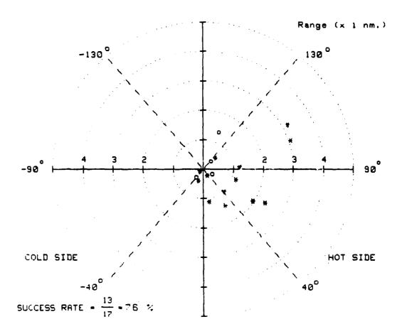
Figure 7. Sample display format for Envelope Recognition: Sparrow AIM 7F -- shows fighter aircraft position at missile fire in terms of range (n.m.) and angle off tail (AOT in degrees) from target. Circles and stars indicate hits and misses, respectively, according to preselected rules for scoring.
