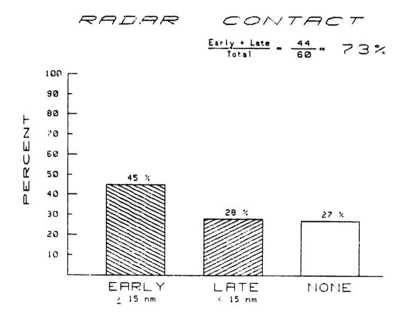
Figure 3. Sample display format for Radar Contact: percent of engagements with early, late and no radar contact
