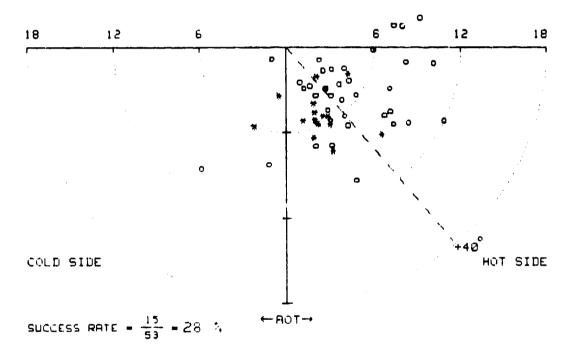
Figure 6. Sample display format for Envelope Recognition: Sidewinder AIM 9G -- shows fighter aircraft position at missile fire in terms of range (x1000 ft.) and angle off tail (AOT in degrees) from target. Circles and stars indicate hits and misses, respectively, according to preselected rules for scoring.
