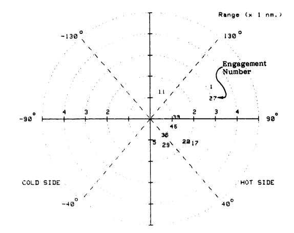
Figure 10. Sample display format for Envelope Recognition (by engagement) for selected missile: shows fighter aircraft fire position in terms of range (n.m.) and angle off tail (AOT in degrees) from target. Numbers refer to engagement number of each shot.
