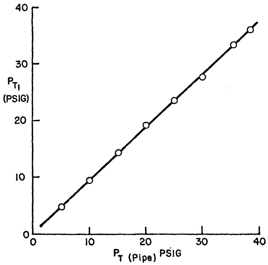
FIGURE 14 VARIATION OF NOZZLE TOTAL PRESSURE WITH TOTAL PRESSURE AT ORIFICE INLET
