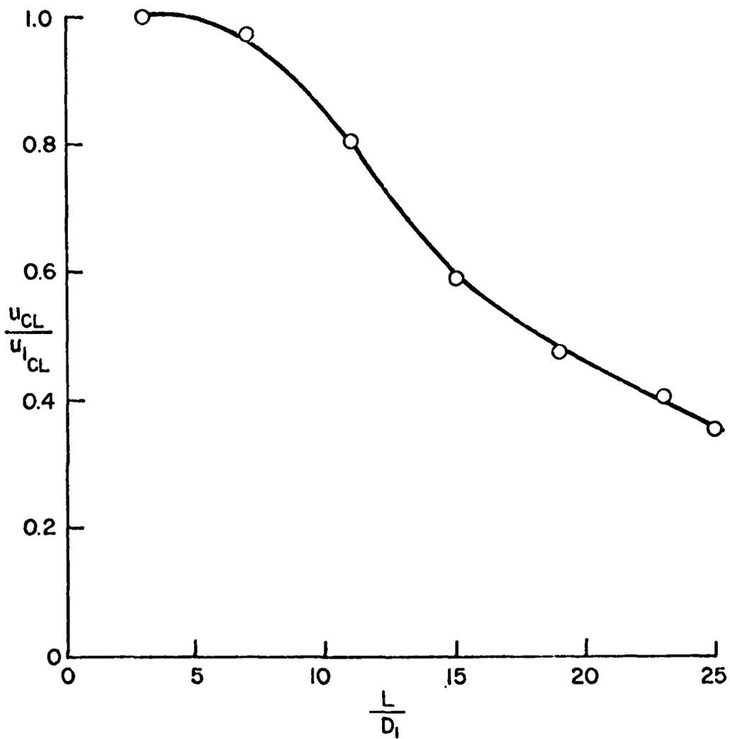
FIGURE 16 CENTERLINE VELOCITY DECAY,
