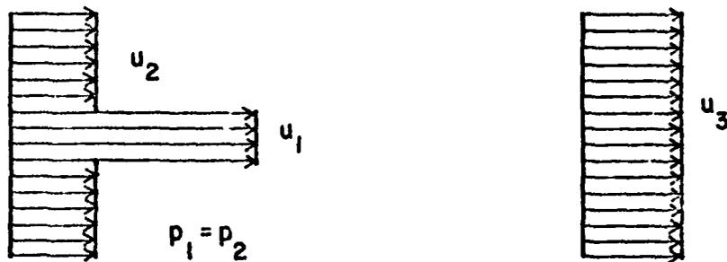
FIGURE 2 STATION DESIGNATION AND IDEAL VELOCITY PROFILES FOR JET PUMP ANALYSIS
