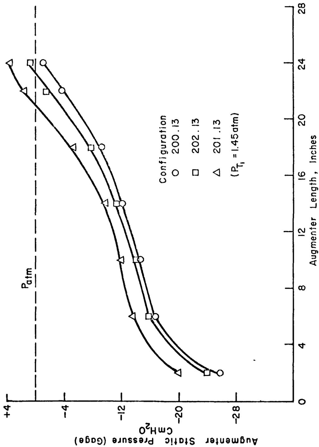
FIGURE 26 AUGMENTER PRESSURE RISE WITH COLANDERS INSTALLED
