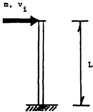
FIG 1-1 Isolated Pile: Cantilever
