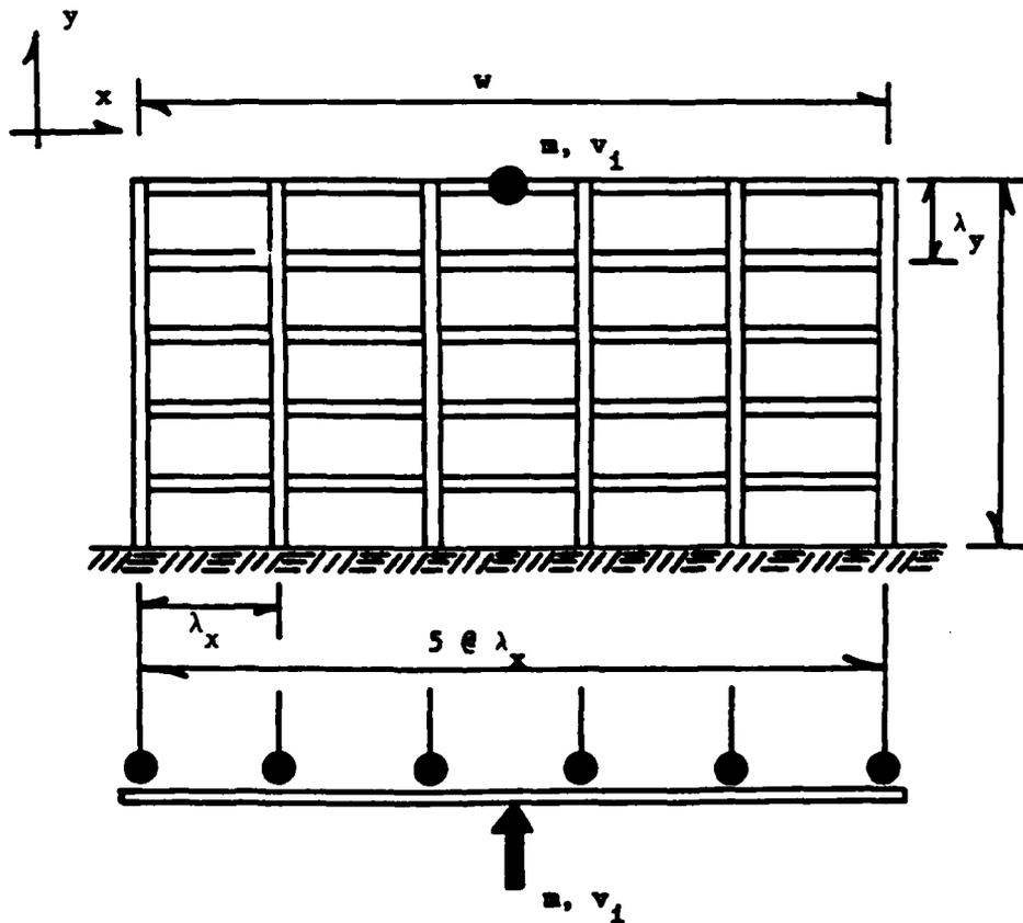
FIG 1-2 Fendering System (Vertical Piles with Horizontal
