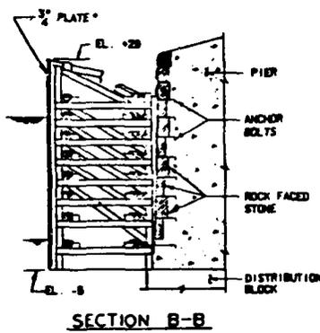
\* EXPOSED METAL PLATES TO HAVE A SPARK-RESISTANT COATING.
