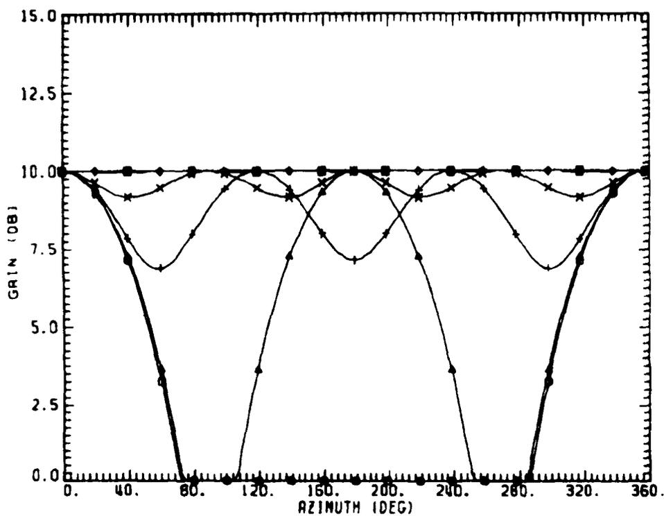
Figure 2. Array gains in uncorrelated receiver noise when  $r/\lambda = 1/8$
