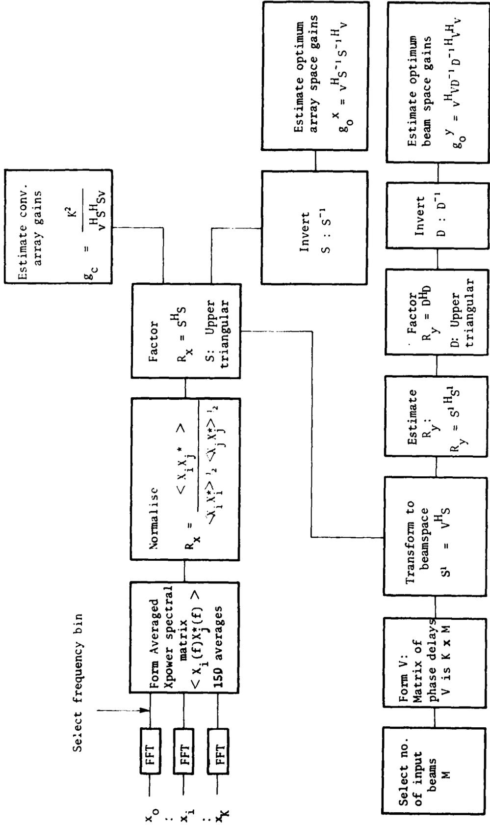
Figure 8. Block diagram for comparison of conventional, array space and beam space array gain estimates
