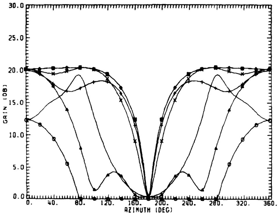
Figure 4. Array gains in uncorrelated receiver noise plus 10 dB interference when  $r/\lambda = 1/8$
