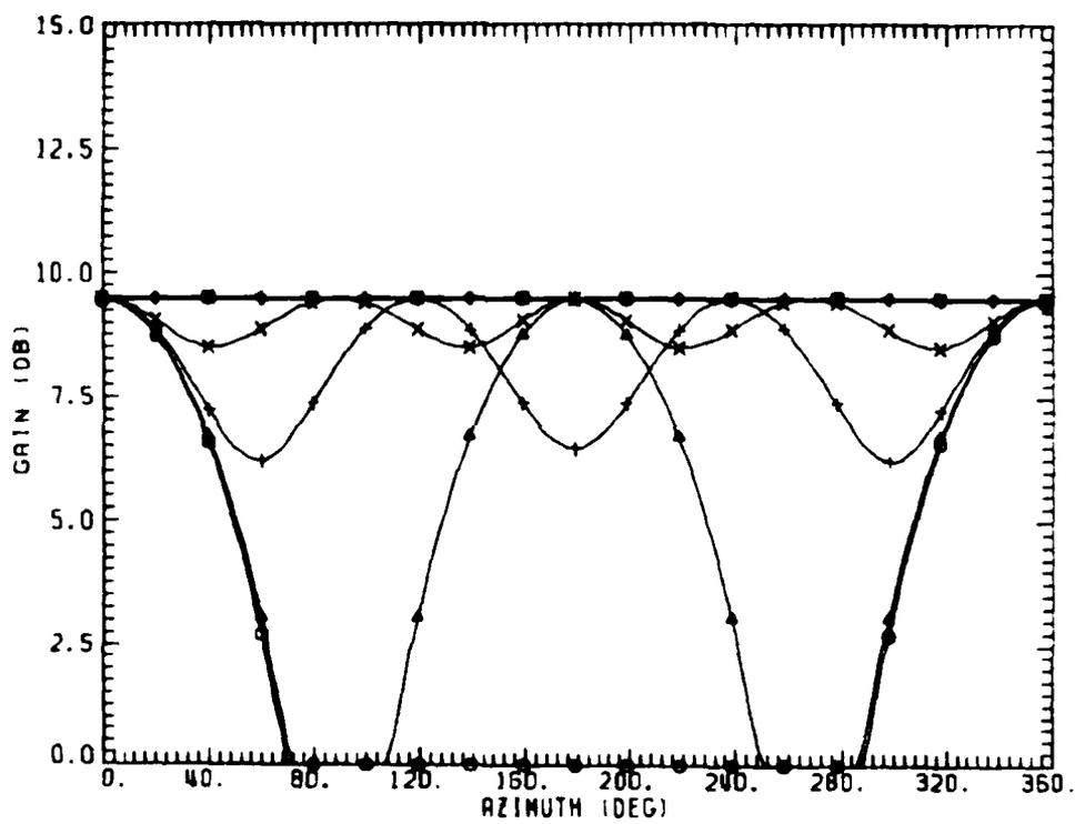
Figure 5. Array gains in isotropic noise when  $r/\lambda = 1/8$
