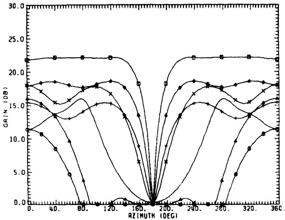
Figure 6. Array gains in isotropic noise plus 10 dB interference when  $r/\lambda = 1/8$
