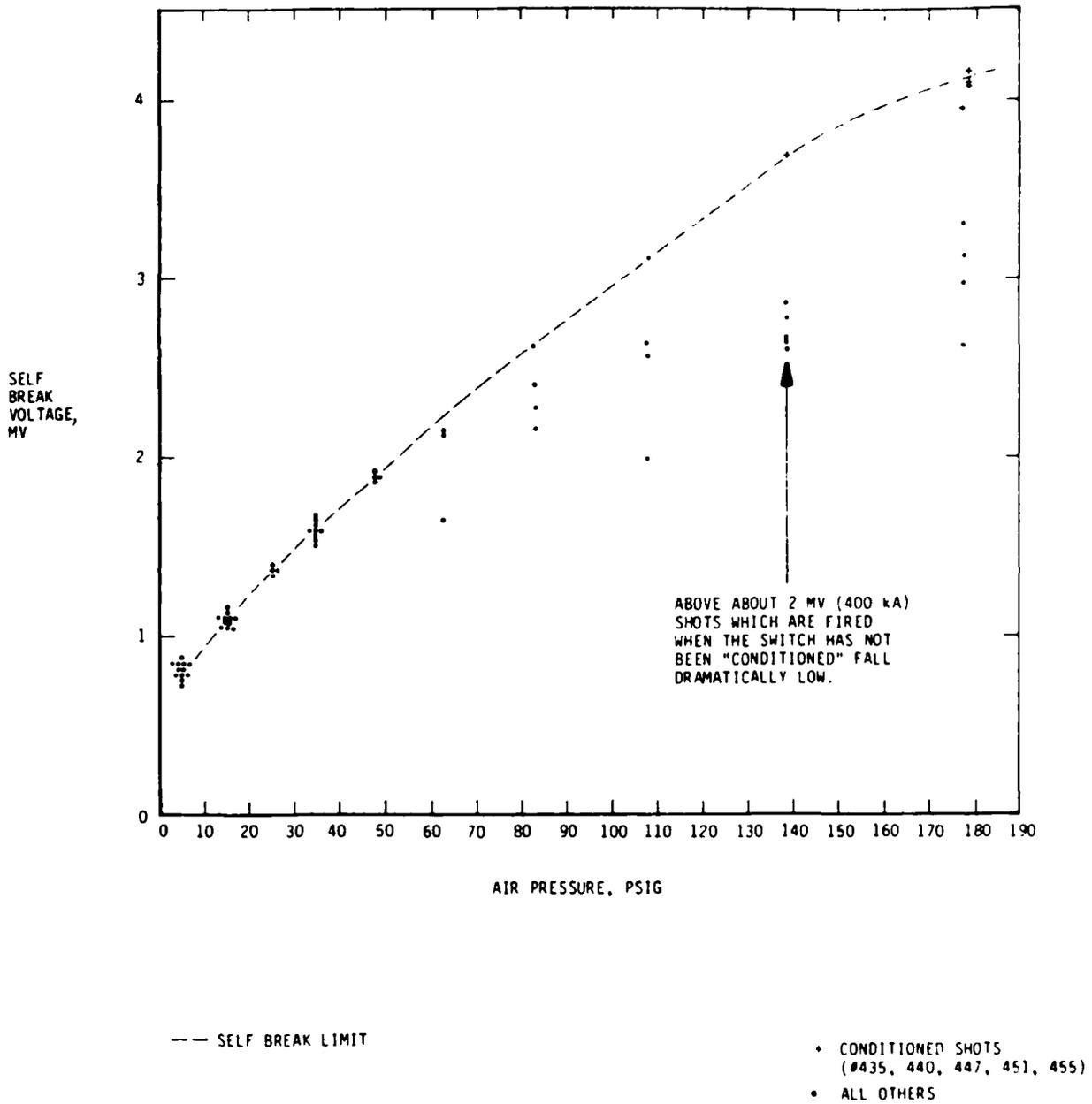
FIGURE 26 DATA FROM TABLE II (12" ELECTRODE PLATE REVERSED)
