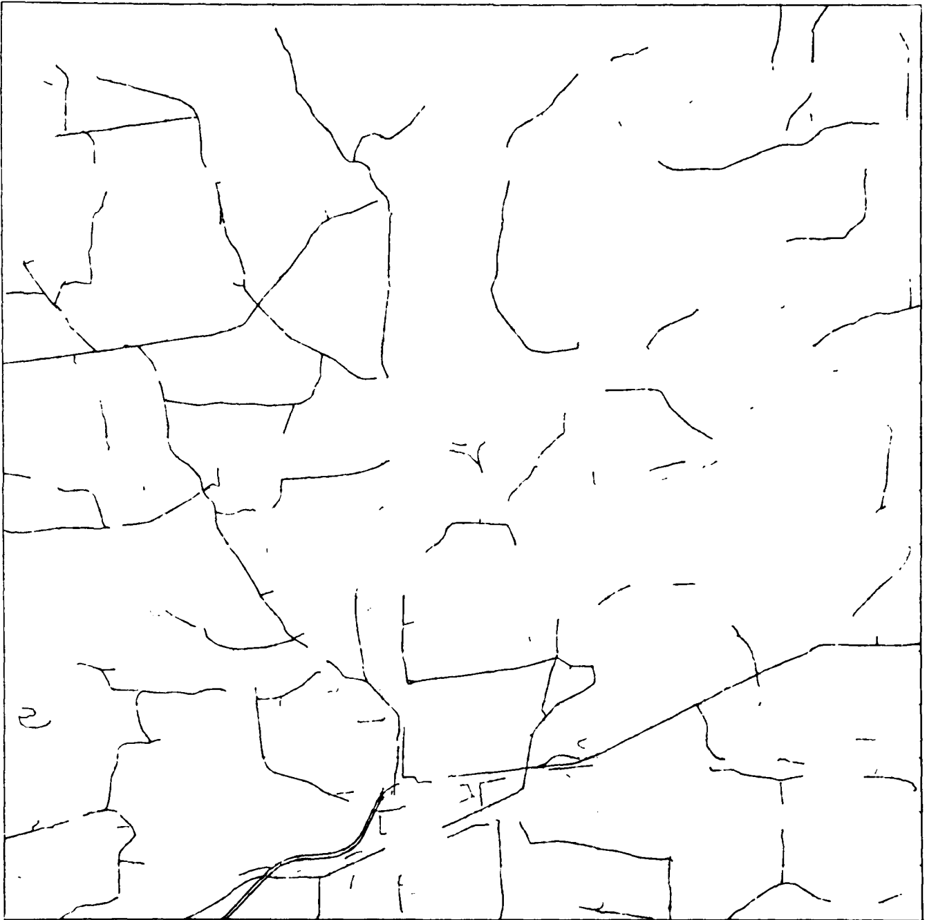
Fig. 8: Extraction result for medium size roads of 3 to 6 pixels.
