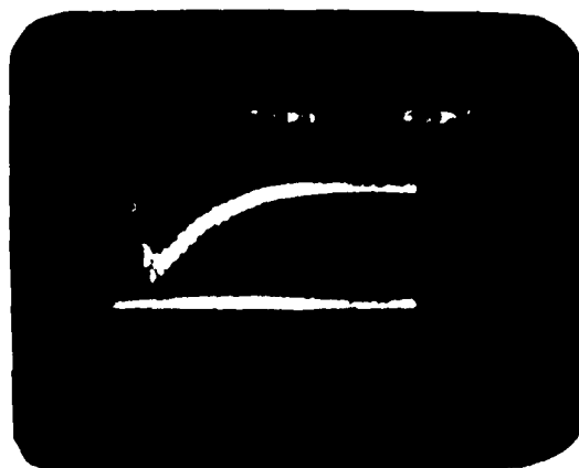
Generator Coil 1 Layer Insulation Pass 8 KV Vertical: 2000 V/div. Horizontal: 500 ns/div.
