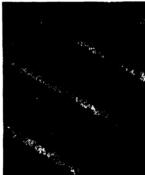
Fig. 2 — Silver L_{\alpha} X-ray intensity map of region shown in Fig. 1. Intensities off lines are background.
