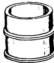
b. Cylinder with Integral Stiffeners
