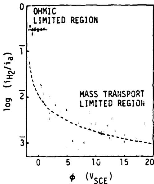
Fig. 2. Ratio of hydrogen current density to anodic current density in ohmic limited and mass transport limited regions for 0.94 M MgCl<sub>2</sub>.
