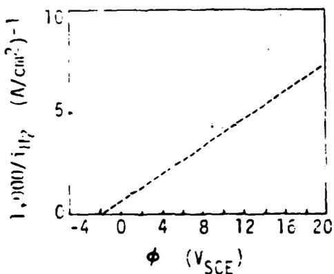
Fig. 3. Plot of reciprocal of hydrogen evolution current density versus potential (Eq. 7) for mass transport limited region with 0.94 M MgCl<sub>2</sub>.
