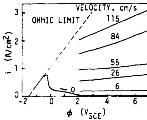
Fig. 4. Effect of electrolyte velocity on current density in mass transport limited region in 4.7 M MgCl<sub>2</sub>; depth = 1.5 mm.
