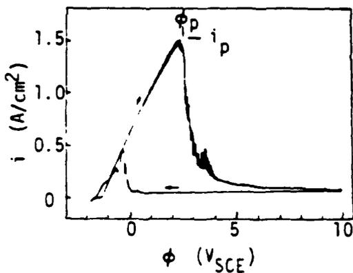
Fig. 1. Potentiodynamic polarization curve for magnesium in 0.94 M MgCl<sub>2</sub>; depth = 2 mm; sweep rate = 1 V/min.
