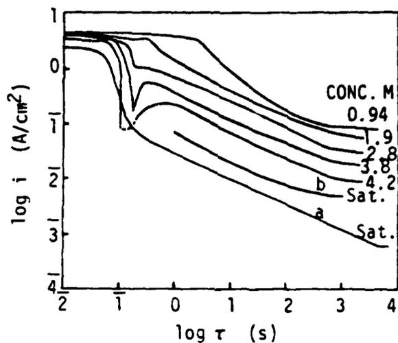
Fig. 5. Current-time transients for Mg in  $\text{MgCl}_2$  solutions at  $\phi = 5.0 \text{ V}_{\text{SCE}}$ ; depth = 0.9 mm; a = cooled from  $30^\circ\text{C}$ , b = cooled from  $50^\circ\text{C}$  to  $21^\circ\text{C}$ .
