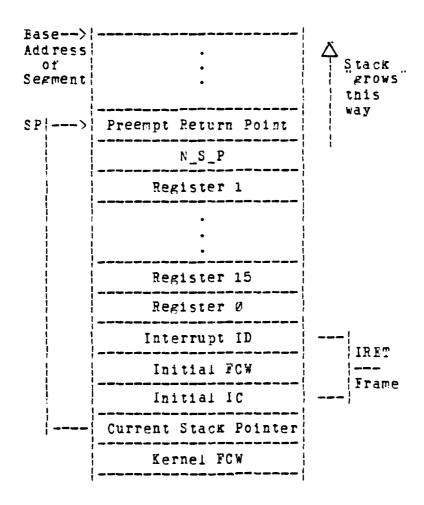
Figure 9. Initial Process Stack
