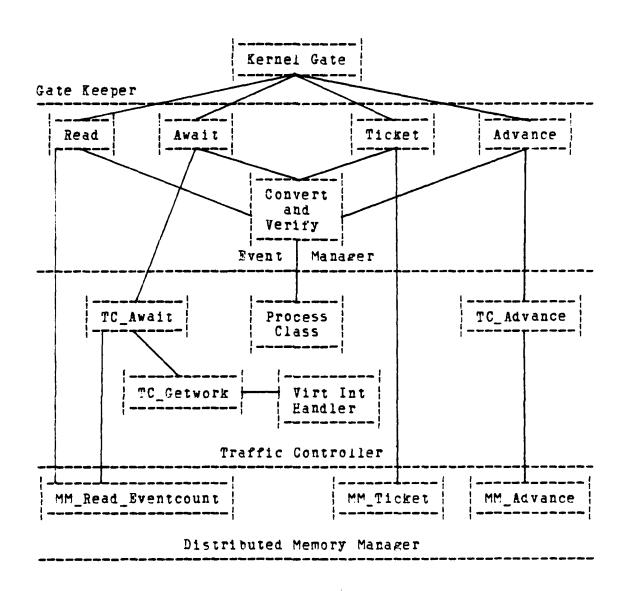
Figure 10. Implementation Module Structure
