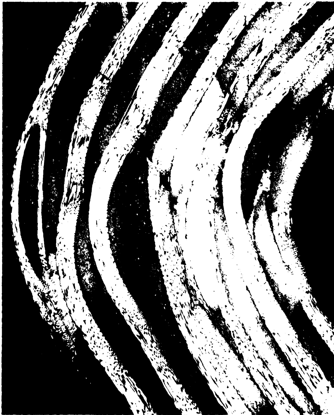
Figure 15.—Photomicrograph #1 of Postformed NTS20-1 Laminate
