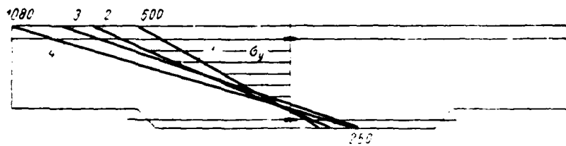
Fig. 72. The dependence of stresses/voltages \sigma_y in the mean section of supporting beam (plate/slab) from the tightening of pins [24]: 1 - all pins are tightened; 2 - are weakened six average/mean horizontal pins; 3 - are weakened all horizontal pins; 4 - are weakened all pins.
