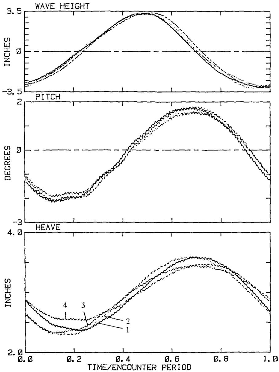
FIGURE 11.2 WAVE ELEVATION, PITCH AND HEAVE, RUN 23,
