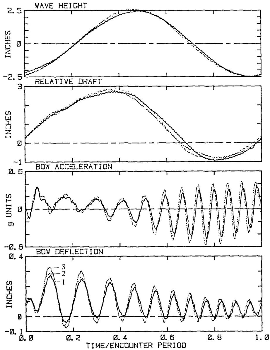
FIGURE 10.3 WAVE ELEVATION, KNUCKLE DRAFT, BOW ACCELERATION AND BOW DEFLECTION, RUN 22
