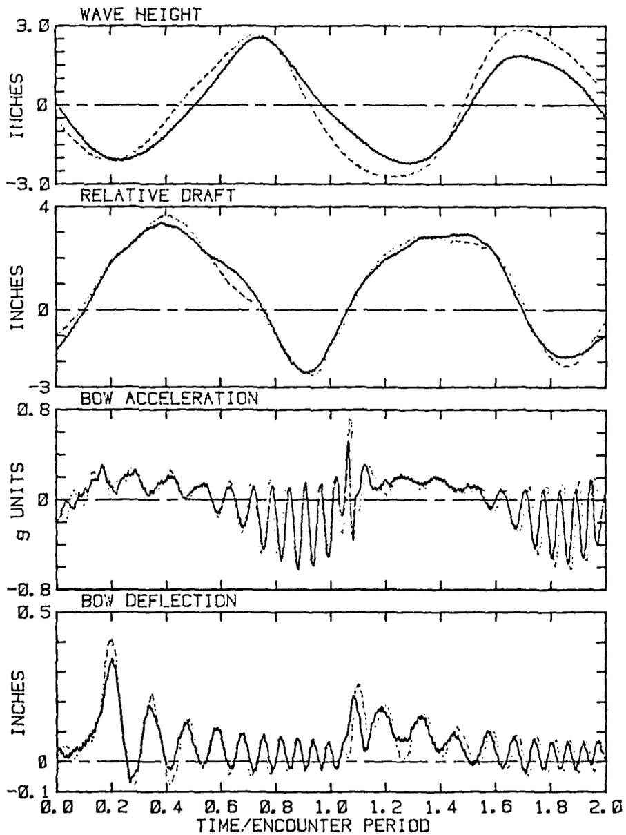
FIGURE 14.3 WAVE ELEVATION, KNUCKLE DRAFT, BOW ACCELERATION AND BOW DISPLACEMENT, RUN 26
