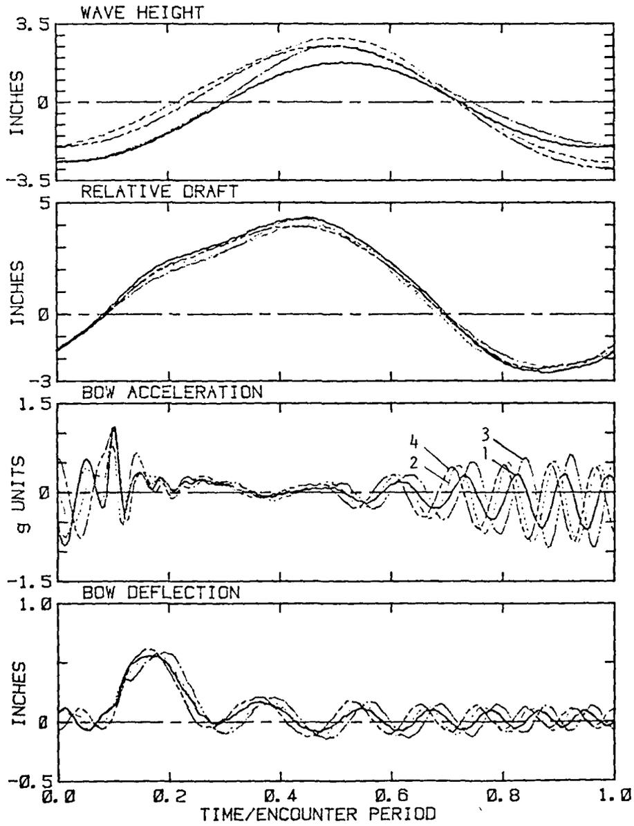
FIGURE 12.3 WAVE ELEVATION, KNUCKLE DRAFT, BOW ACCELERATION AND BOW DISPLACEMENT, RUN 25
