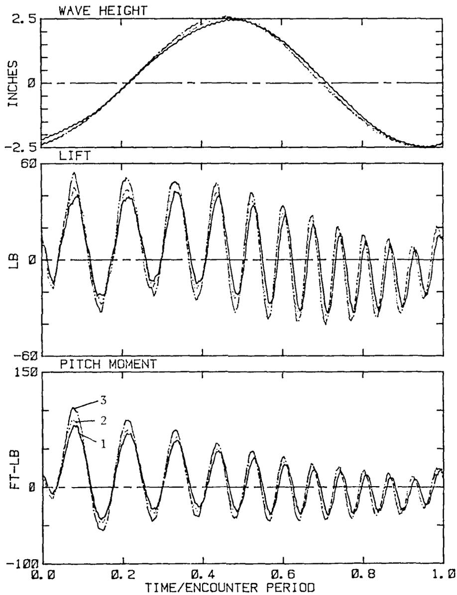
FIGURE 10.1 WAVE ELEVATION, SHEAR AND BENDING MOMENT, RUN 22
