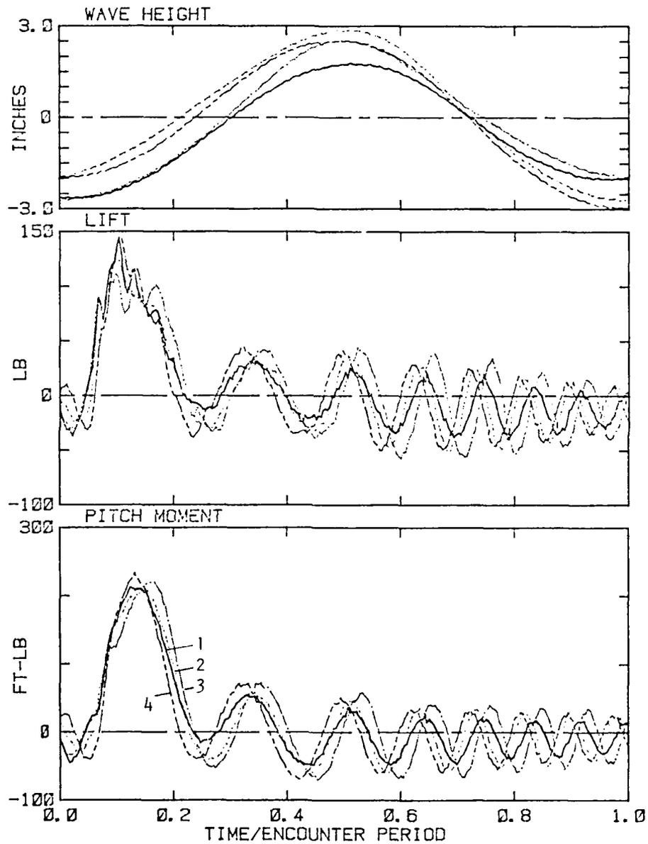
FIGURE 12.1 WAVE ELEVATION, SHEAR AND BENDING MOMENT, RUN 25.
