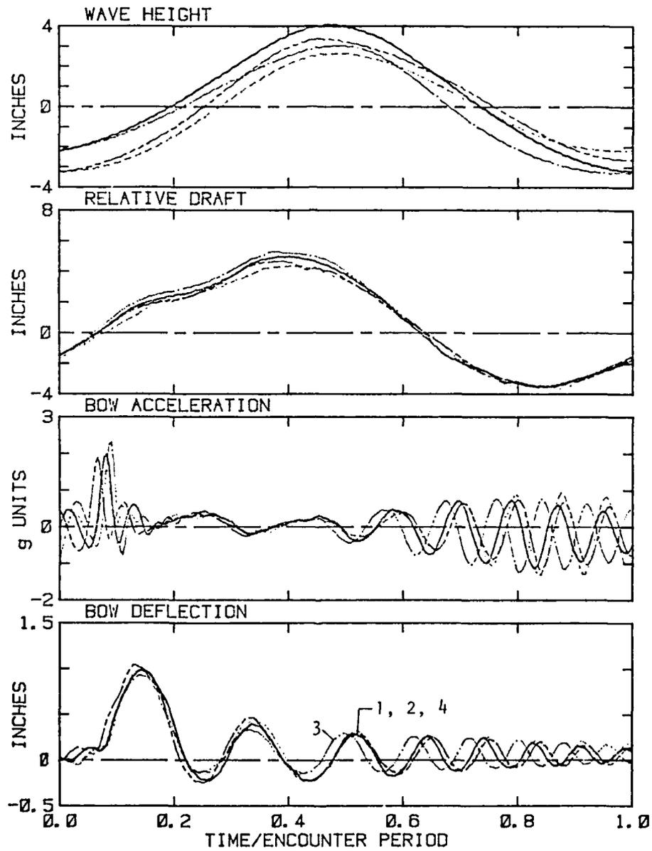
FIGURE 13.3 WAVE ELEVATION, KNUCKLE DRAFT, BOW ACCELERATION AND BOW DISPLACEMENT, RUN 24
