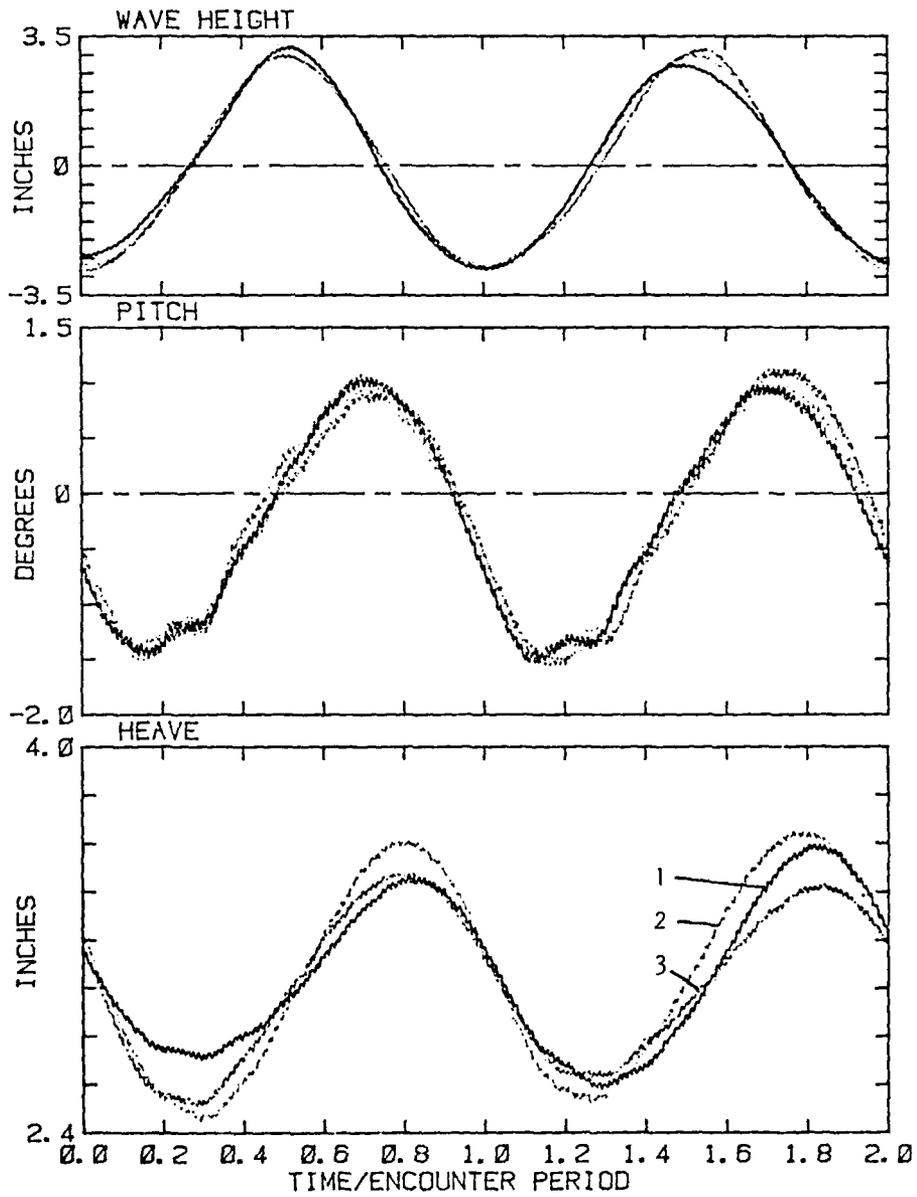
FIGURE 9.2 WAVE ELEVATION, PITCH AND HEAVE, RUN 21, MODEL SPEED ZERO, ENCOUNTER PERIOD 1.31 SECONDS, WAVE HEIGHT 5.67 INCHES
