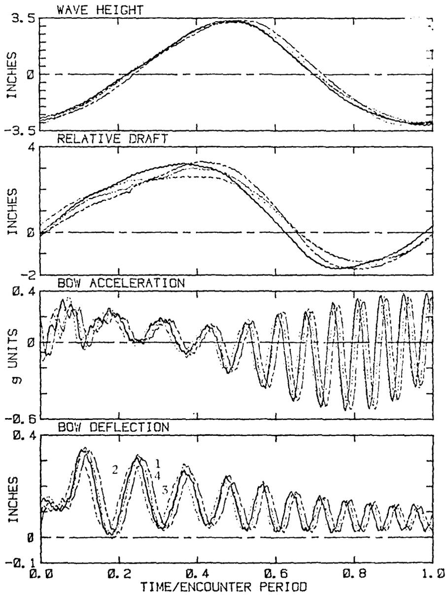
FIGURE 11.3 WAVE ELEVATION, KNUCKLE DRAFT, BOW ACCELERATION AND BOW DISPLACEMENT, RUN 23
