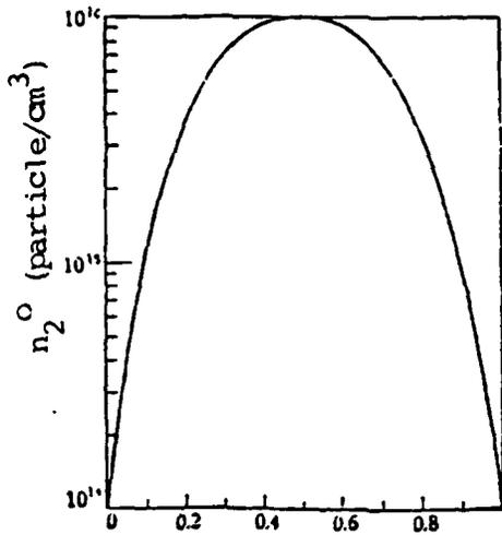
Figure 4.1. The variation of  $n_2^0$  with  $\frac{u}{L_1}$  at inlet of optical chamber.
