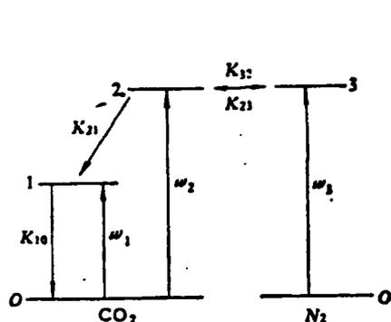
Figure 2. Energy levels of the  $\text{CO}_2$ - $\text{N}_2$  laser system and relaxation processes.
