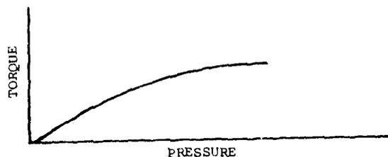
FIGURE 16 IDEAL PRESSURE VS TORQUE RELATIONSHIP
