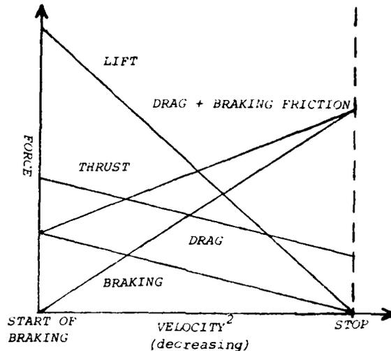
FIGURE 2 VARIATION OF FORCES DURING LANDING ROLL.
