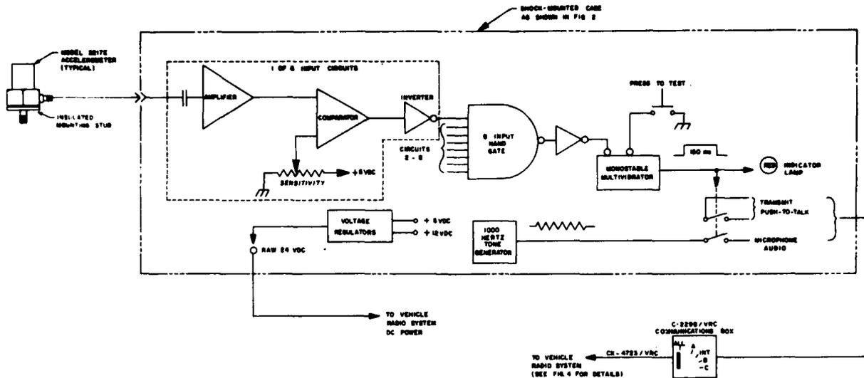
Figure 3. Hit detector signal conditioning equipment.
