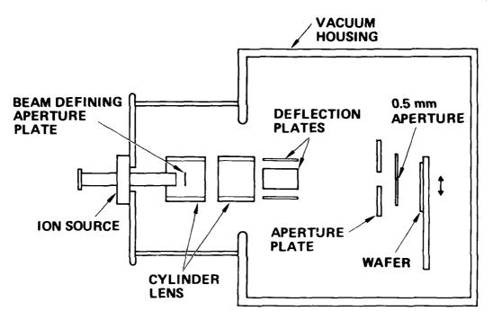
Figure 1. Schematic of the low-current-density exposure apparatus.
