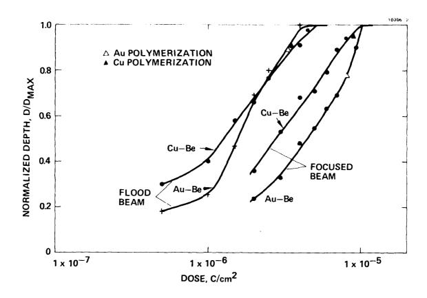
Figure 2. Exposure curves for the beryllium alloys.
