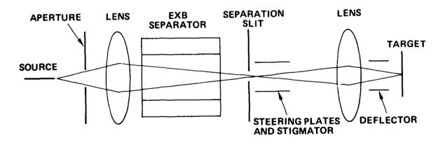
Figure 6. Comparison of required column components with and without mass separation.
