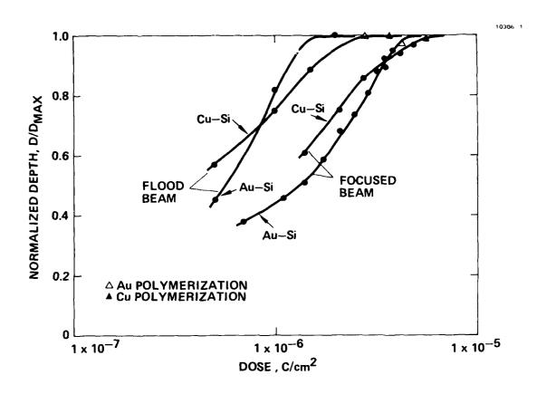
Figure 3. Exposure curves for the silicon alloys.
