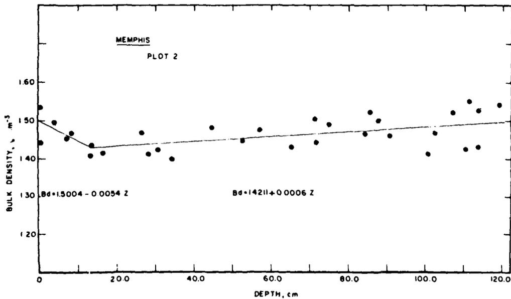
Figure 22 The bulk density - depth relationship for a Memphis soil.
