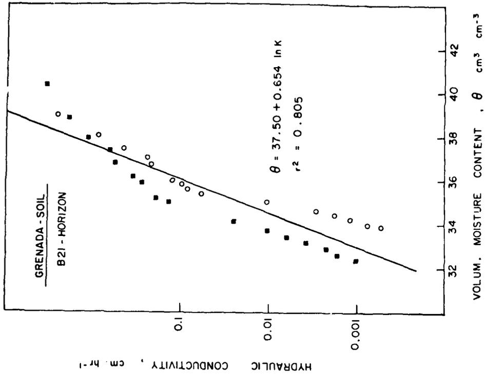
Figure 11 In situ hydraulic conductivity vs volumetric water content for the B<sub>21</sub>-horizon of the Grenada soil.
