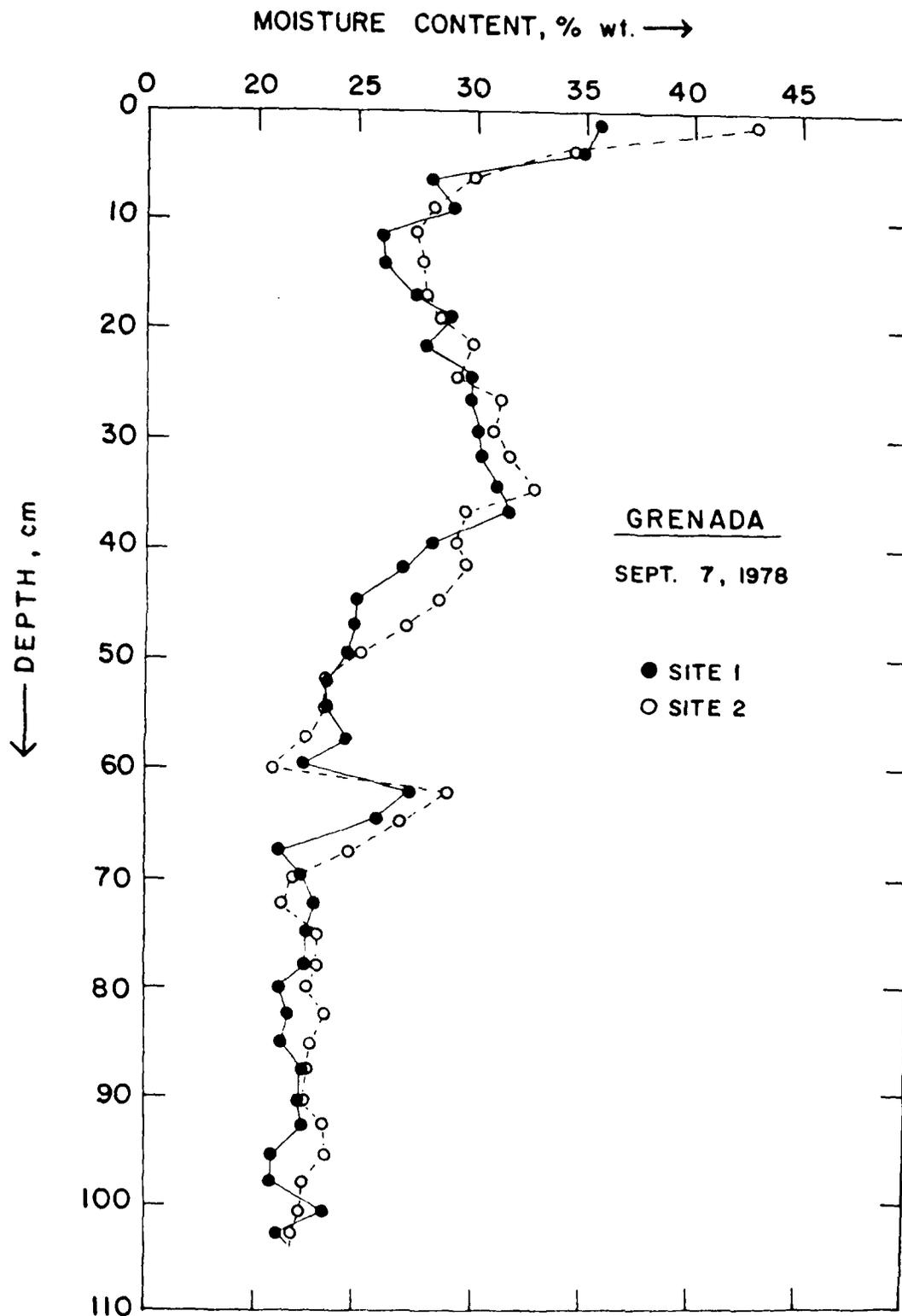
Figure 4 Gravimetric determinations of soil water content as a function of depth.
