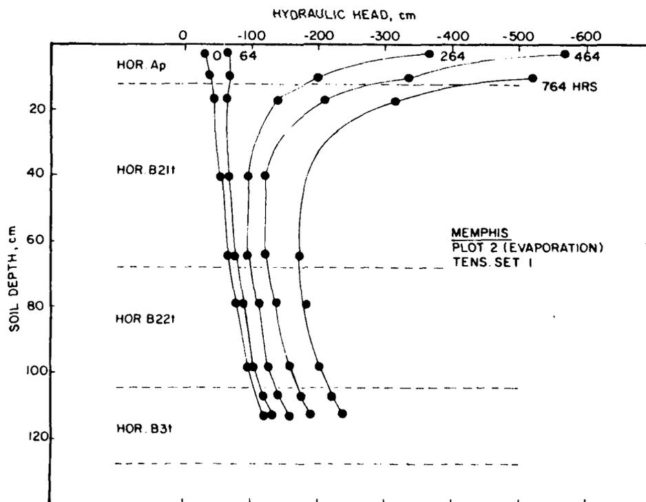
Figure 24 Pressure head and hydraulic head relationships during simultaneous drainage and evaporation for a Memphis soil.
