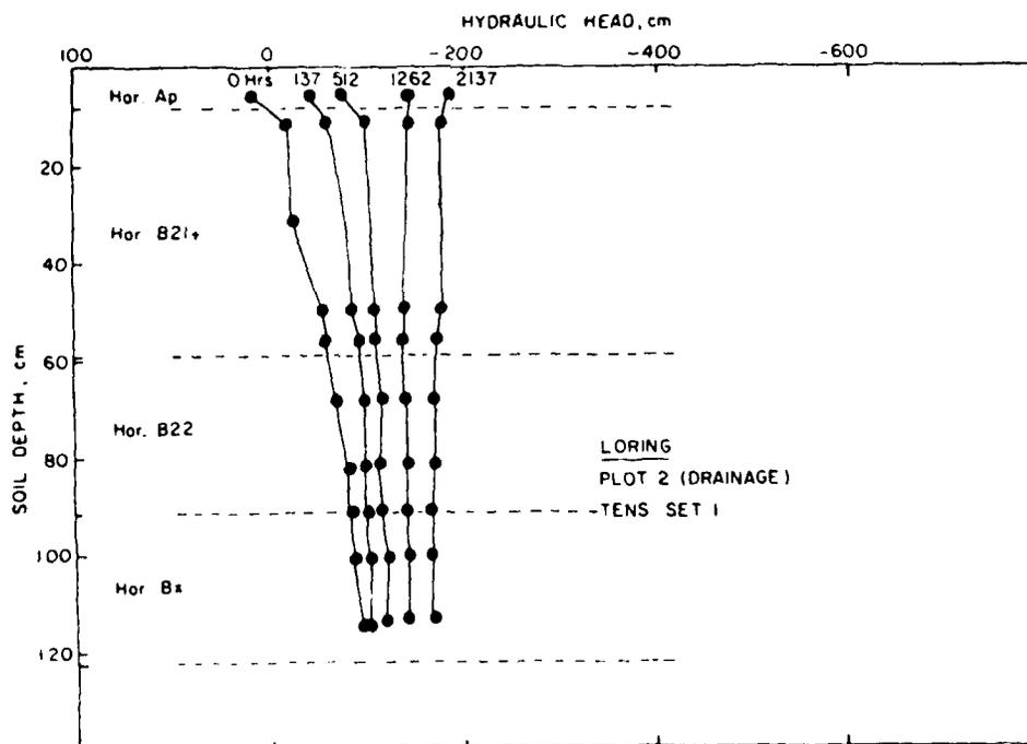
Figure 16 Pressure head and hydraulic head relationships during drainage for a Loring soil (Plot 2).
