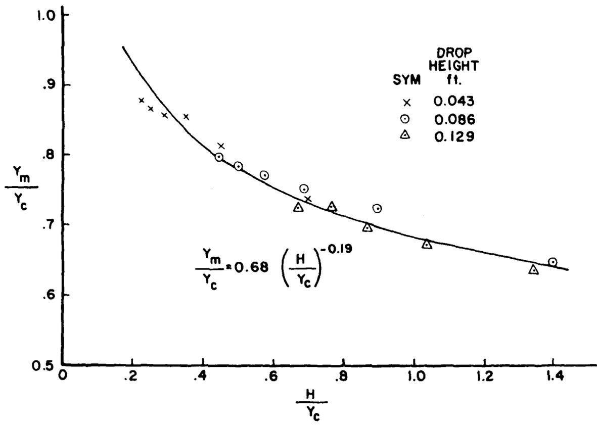
Figure 13 Plot of Ratio of Minimum Depth to Critical Depth Versus Relative Drop Height.
