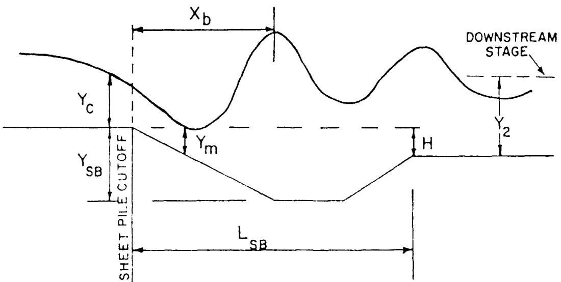
Figure 19. Schematic of an Hydraulic Low Drop Structure.
