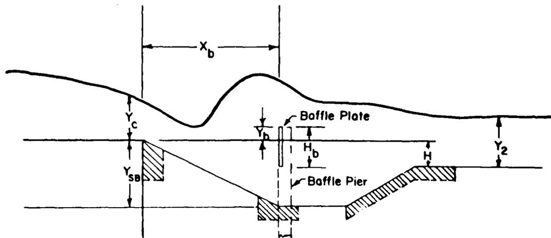
Figure 15 Basin Dimensions and Riprap Placement.
