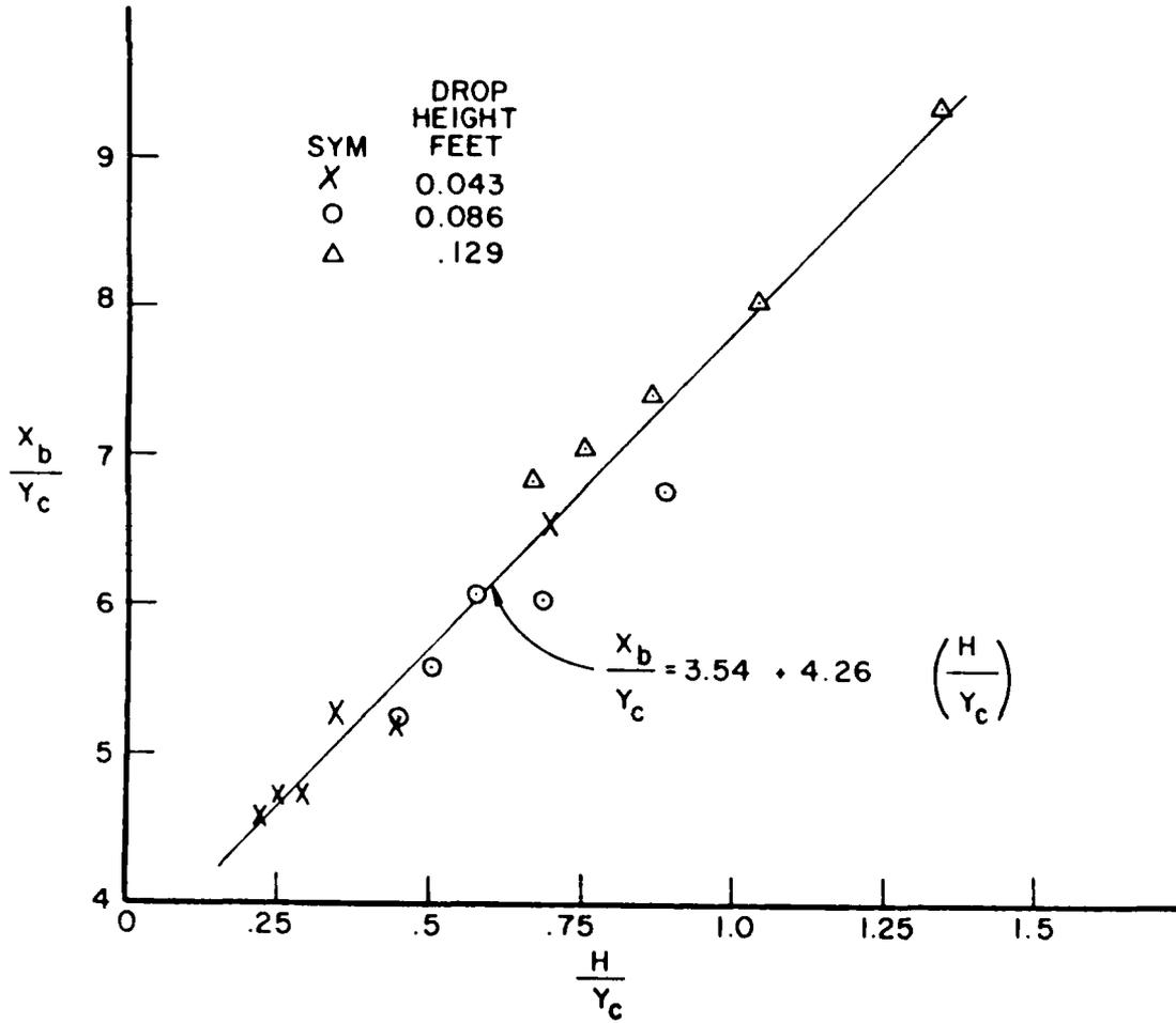
Figure 14 Plot of Ratio of Distance to Crest of First Undulation to Critical Depth Versus Relative Drop Height.
