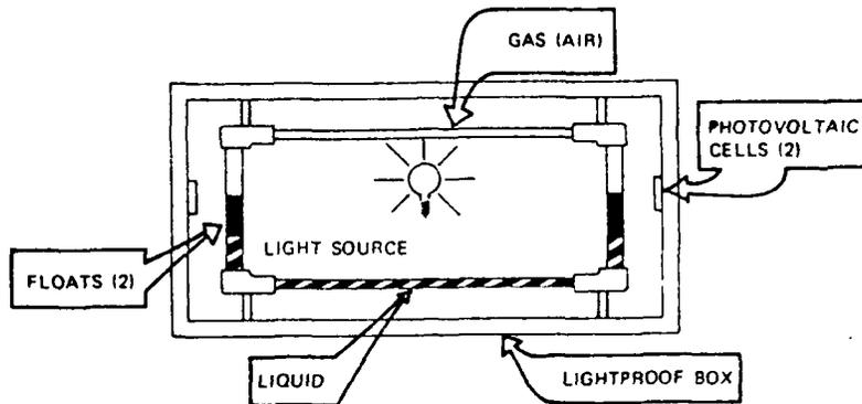
Figure 3 - Angle Sensor Schematic
