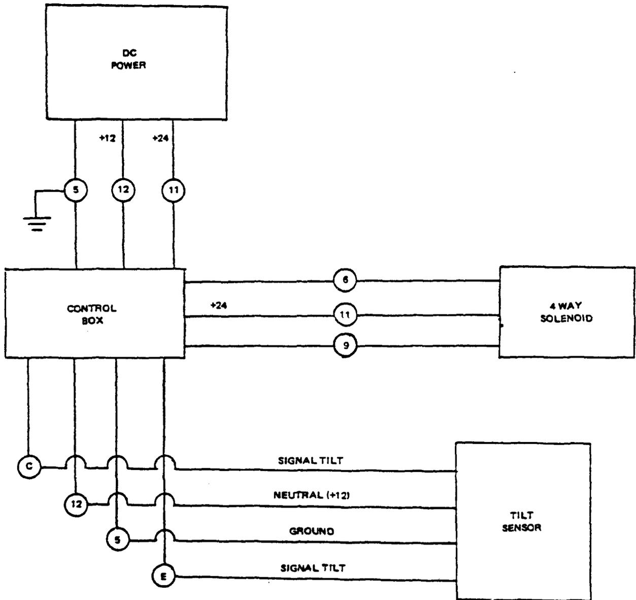
TILT ANGLE ELECTRICAL SCHEMATIC
