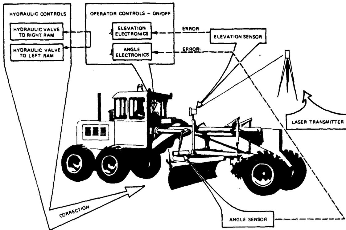
Figure 1 - Automatic Blade Control System Schematic
