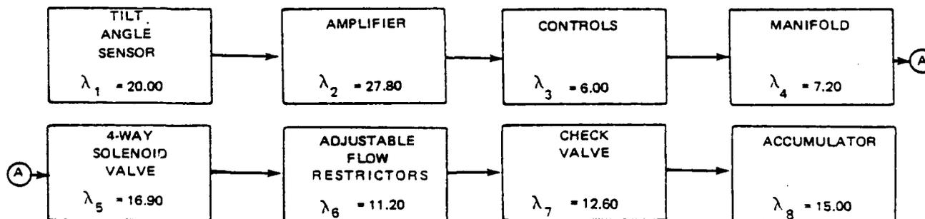
$$R = e^{-\lambda t} \quad \lambda = \sum \lambda_i = 116.7 \text{ FAILURES}/10^6 \text{ HOURS}$$
