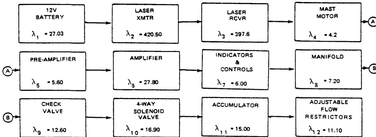
$$R = e^{-\lambda t} \quad \lambda = \sum \lambda_i = 951.6 \text{ FAILURES}/10^6 \text{ HOURS}$$
